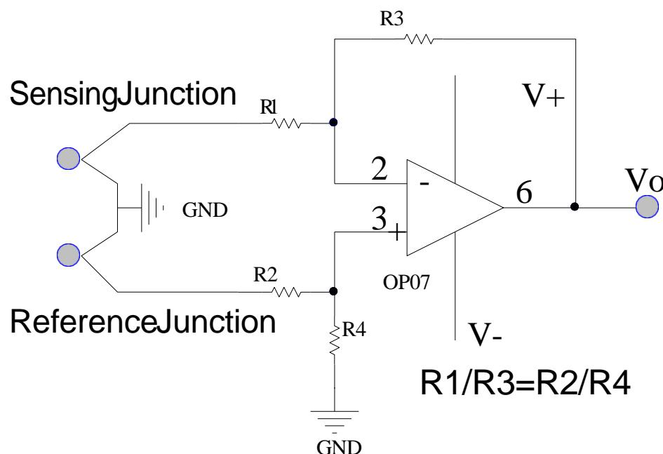
**High stability thermocouple amplification**
