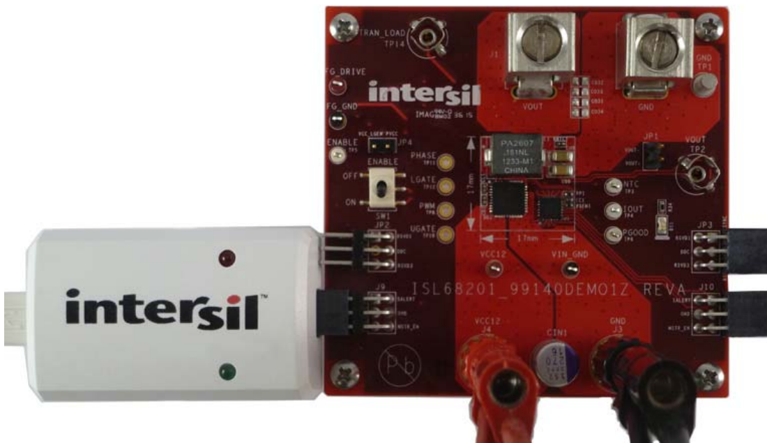
FIGURE 5. ISL68201-99140DEMO1Z DEMONSTRATION KIT SET-UP
