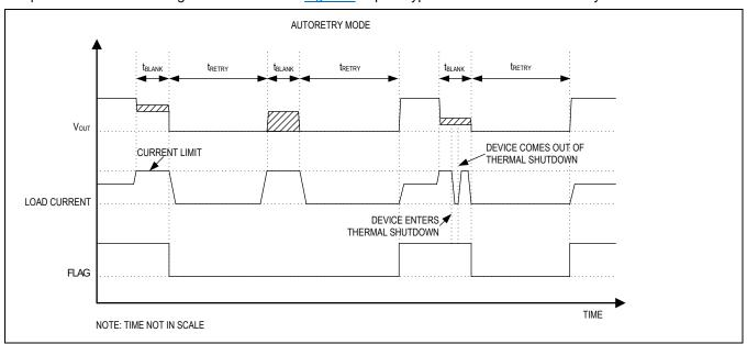
Figure 3. Autoretry Fault-Timing Diagram
