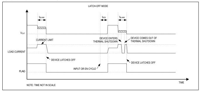
Figure 5. Latch-Off Fault-Timing Diagram
