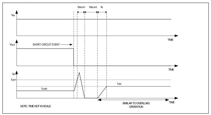
Figure 6. Fast Overcurrent Trip Timing Diagram
