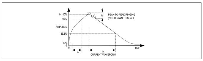
Figure 10. Human Body Current Waveform
