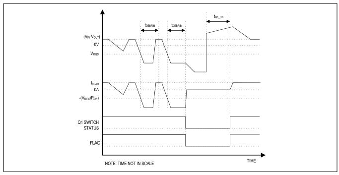
Figure 7. Slow Reverse-Current Fault-Timing Diagram
