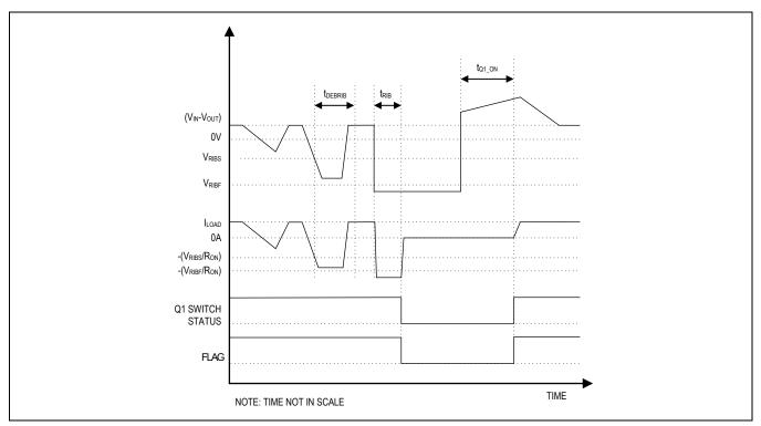
Figure 8. Fast Reverse-Current Fault-Timing Diagram
