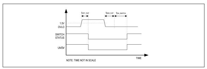
Figure 1. Overvoltage-Fault Timing Diagram
