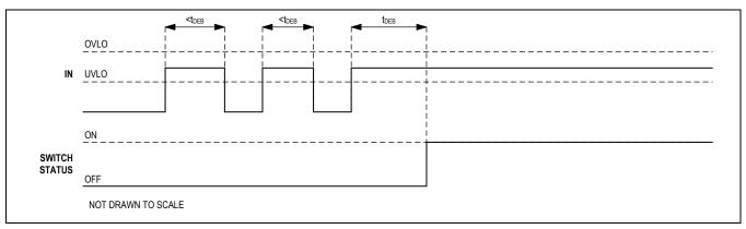
Figure 2. Debounce Timing Diagram
