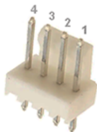
Pin 3,4: V+, Pin 1,2:V-
