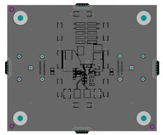
Figure 4-2. Top Layer Routing
