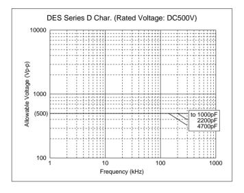
approximately to the allowable voltage for a sine wave whose fundamental frequency is twice as large as that of the rectangular wave or pulse wave.
