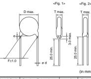
[Bulk] Vertical Crimp Long (Fig. 1) Straight Long (Fig. 2)
