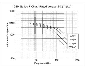
to the allowable voltage for a sine wave whose fundamental frequency is twice as large as that of the rectangular wave or pulse wave. This allowable voltage, however, varies depending on the voltage and current waveforms. Therefore, you are requested to make sure that the selfheating temperature is not higher than the value specified in Table 1.
