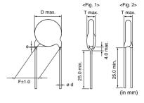
[Bulk] Vertical Crimp Long (Fig. 1) Straight Long (Fig. 2)
