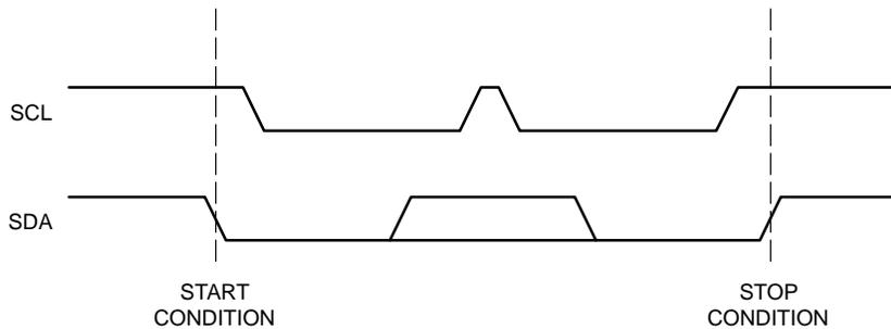
Figure 2. Start/Stop Timing
