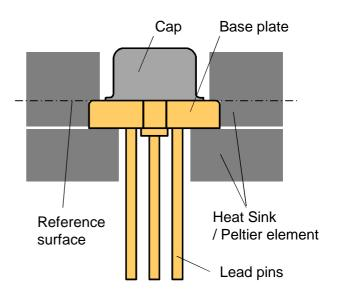
Fig.2 Mounting example of to56 package
