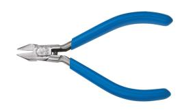
These Electronics Pliers are the smallest diagonal-cutter Klein offers for close quarter work. They feature a miniature jaw for maximum visibility in tight spaces. The sharp, pointed, tapered nose allows for precise tip cutting. The short jaws and semi-flush, beveled cutting knives permit close cutting of wire. Made of the finest U.S. steel alloy and induction hardened for long life.
