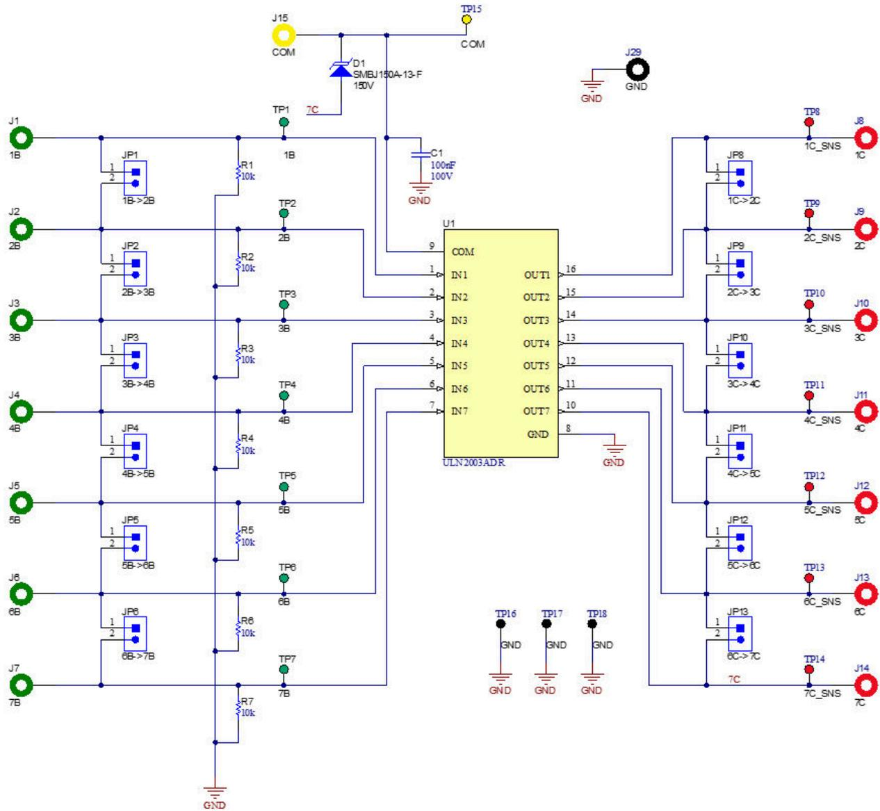
Figure 3-1. ULN2003ADEVM Schematic Drawing
