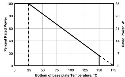
Derating (thermal resistance): 0.23W/°C (4.28°C/W). The case temperature is to be used for purposes of establishing the applied power limit. The case temperature measurement must be made with a thermocouple contacting the center of the component mounted on the designed heat sink. Thermal grease should be applied properly.
