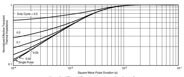
Normalized Thermal Transient Impedance, Junction-to-Case
