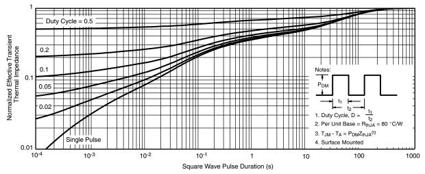
Normalized Thermal Transient Impedance, Junction-to-Ambient
