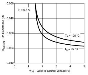
On-Resistance vs. Gate-to-Source Voltage
