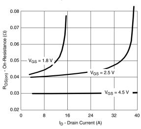
On-Resistance vs. Drain Current and Gate Voltage
