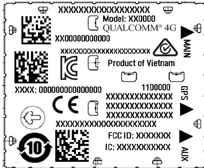
Figure 6-3: Unit Product Marking Example—Laser-etched, Typical Representation (Not to scale. Contents will vary by SKU.)
