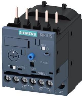
Overload relay 0.32...1.25 A Electronic For motor protection Size S00, Class 10E
