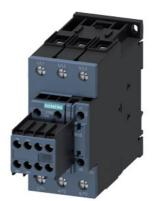
power contactor, AC-3 40 A, 18.5 kW / 400 V 2 NO + 2 NC, AC / DC 84-155 V, with varistor, 3-pole, Size S2, screw terminal
