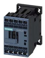
Contactor relay, 3 NO + 1 NC, 110 V AC, 50 / 60 Hz, with full-wave rectifier, Size S00, Spring-type terminal
