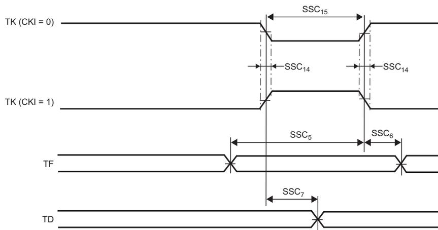
**Figure 54-24: SSC Receiver RK and RF as Input**
