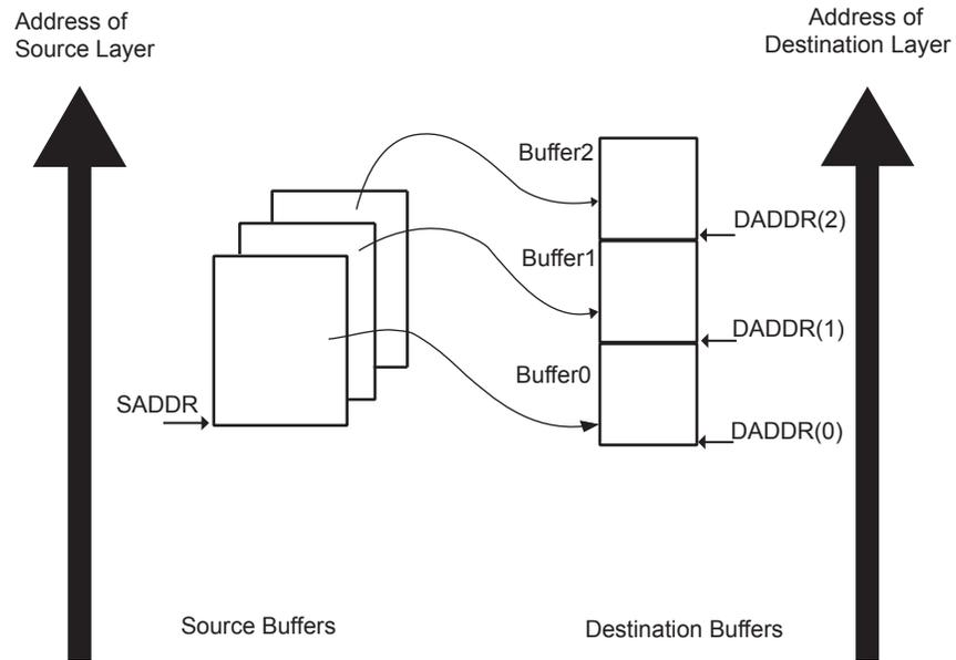
**Figure 31-15: DMAC Transfer Replay Mode is Enabled for the Source and Contiguous Destination Address**
