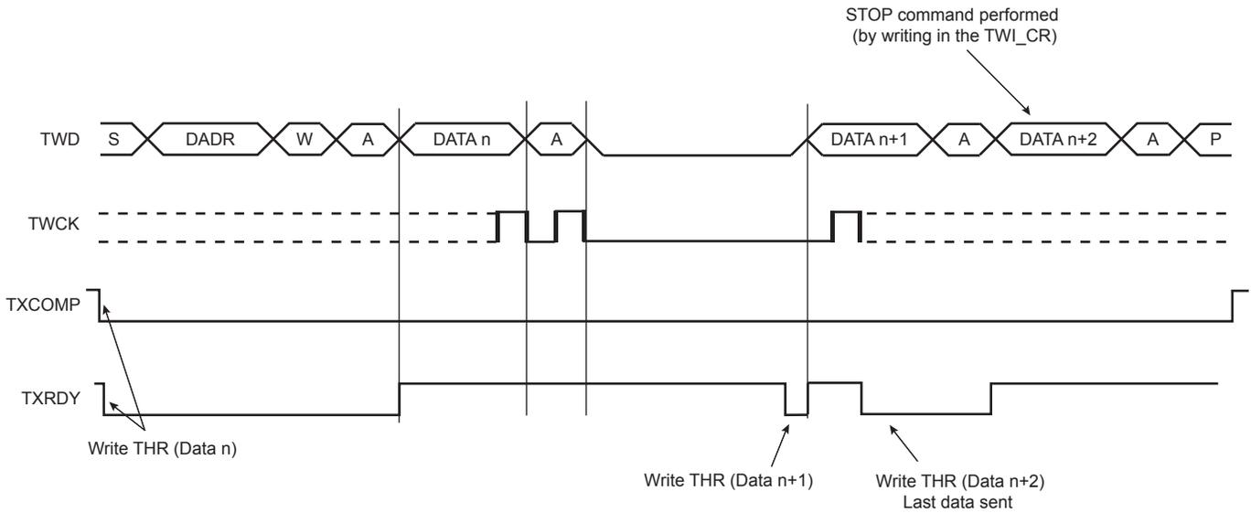
**Figure 40-6: Master Write with One Byte Internal Address and Multiple Data Bytes**
