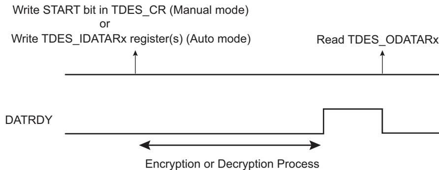
If the user does not want to read the output data registers between each encryption/decryption, the DATRDY flag will not be cleared. If the DATRDY flag is not cleared, the user will not be informed of the end of the encryptions/decryptions that follow.
