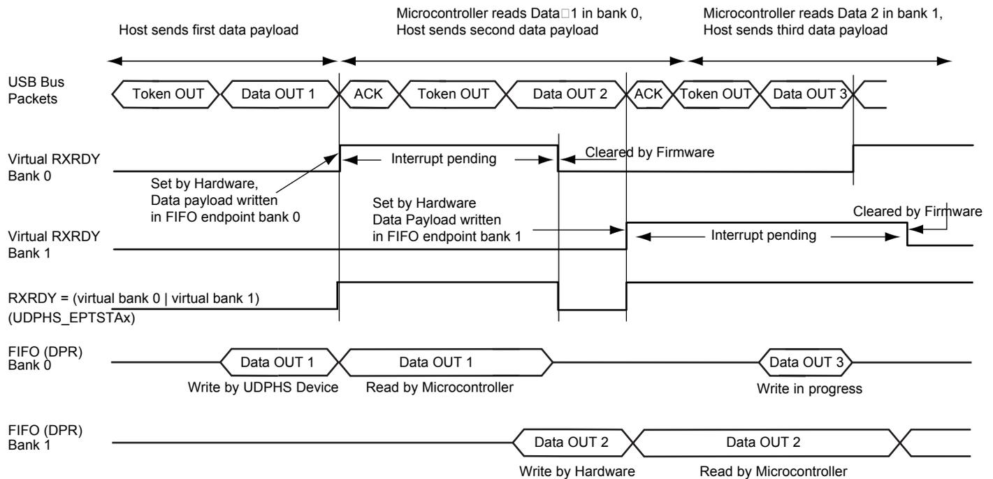
• High Bandwidth Isochronous Endpoint OUT
