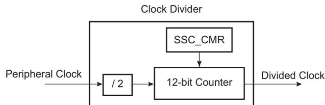
The peripheral clock divider is determined by the 12-bit field DIV counter and comparator (so its maximal value is 4095) in the Clock Mode Register (SSC\_CMCR), allowing a peripheral clock division by up to 8190. The Divided Clock is provided to both the Receiver and Transmitter. When this field is programmed to 0, the Clock Divider is not used and remains inactive.
