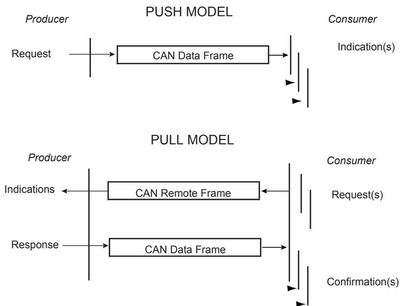
In Pull Mode, a consumer transmits a remote frame to the producer. When the producer receives a remote frame, it sends the answer accepted by one or many consumers. Using transmit and receive mailboxes, a consumer must dedicate two mailboxes, one in Transmit Mode to send remote frames, and at least one in Receive Mode to capture the producer's answer. The same structure is applicable to a producer: one reception mailbox is required to get the remote frame and one transmit mailbox to answer.
