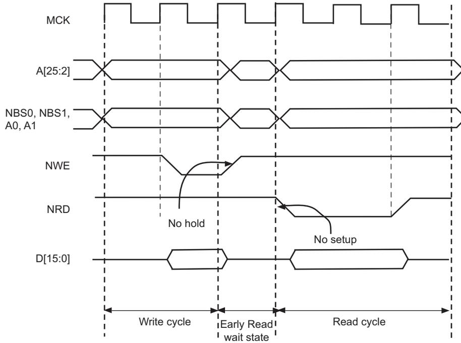
**Figure 30-15: Early Read Wait State: NCS Controlled Write with No Hold Followed by a Read with No NCS Setup**
