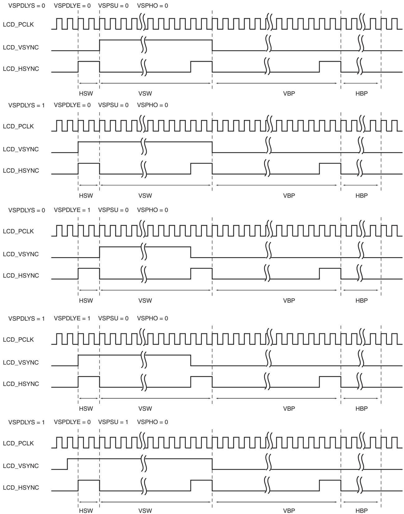
**Figure 32-17: Vertical Synchronization Timing (part 2)**
