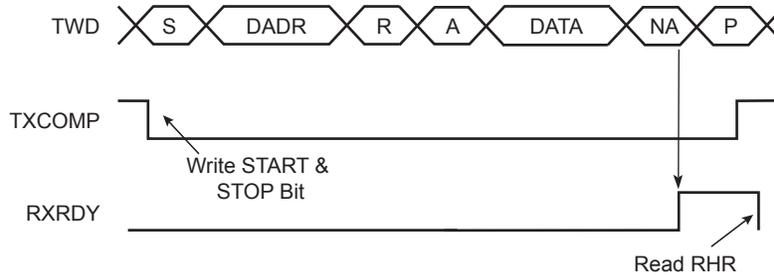
**Figure 40-8: Master Read with Multiple Data Bytes**
