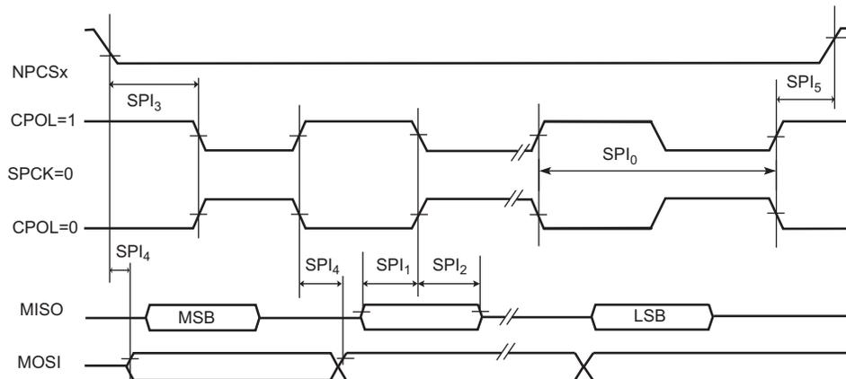
**Figure 54-34: USART SPI Slave Mode (Mode 1 or 2)**
