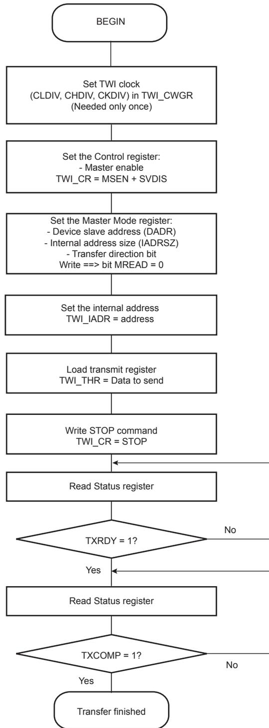
Figure 40-16: TWI Write Operation with Multiple Data Bytes with or without Internal Address
