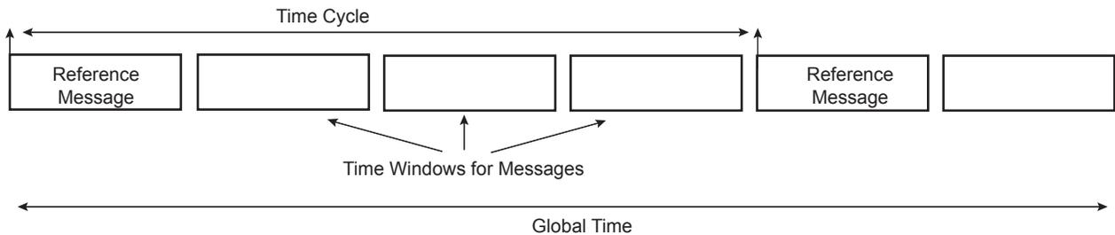
Time Trigger Mode is enabled by setting the TTM field in the CAN\_MR. In Time Triggered Mode, as in Timestamp Mode, the CAN\_TIMESTP field captures the values of the internal counter, but the MTIMESTAMP fields in the CAN\_MSRx registers are not active and are read at 0.
