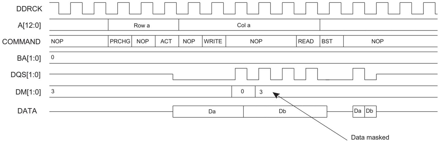
**Figure 29-8: SINGLE Write Access Followed by a Read Access, DDR2-SDRAM Devices**
