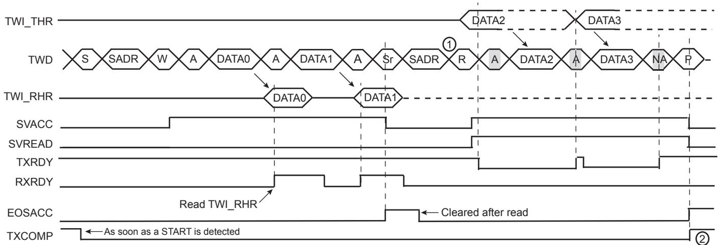
**Note 1:** In this case, if TWI\_THR has not been written at the end of the read command, the clock is automatically stretched before the ACK.
