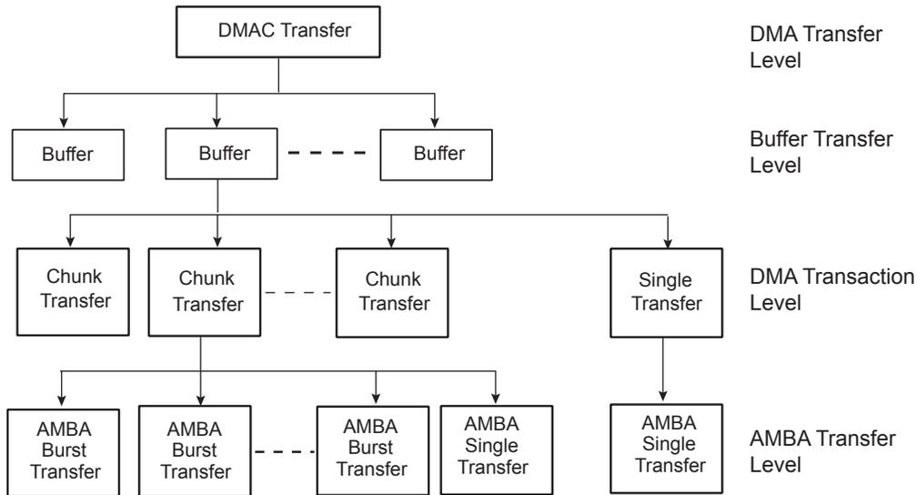
**Figure 31-3: DMAC Transfer Hierarchy for Memory**
