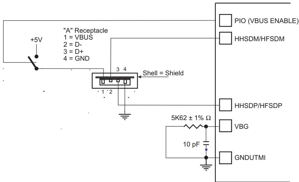
**Figure 56-3: Typical USB High Speed Device Connection**
