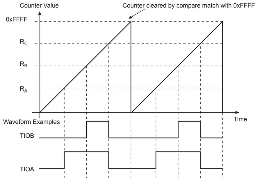
**Figure 47-8: WAVSEL = 00 with Trigger**
