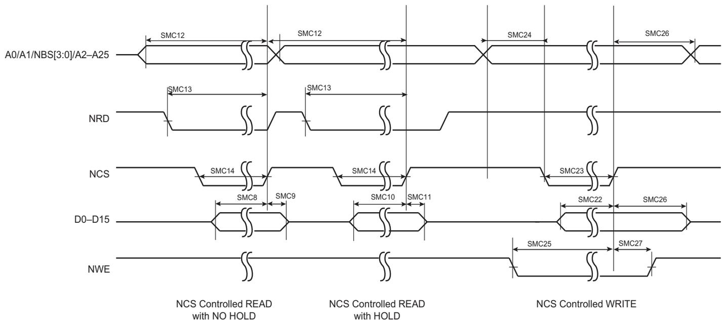
**Figure 54-10: SMC Timings - NRD Controlled Read and NWE Controlled Write**
