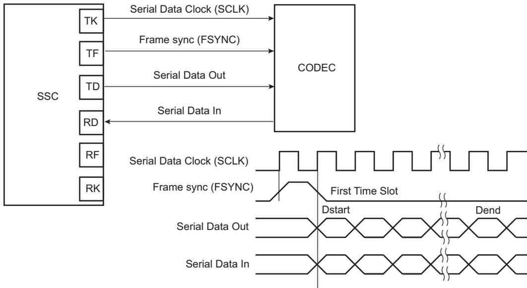
**Figure 41-5: Time Slot Application Block Diagram**
