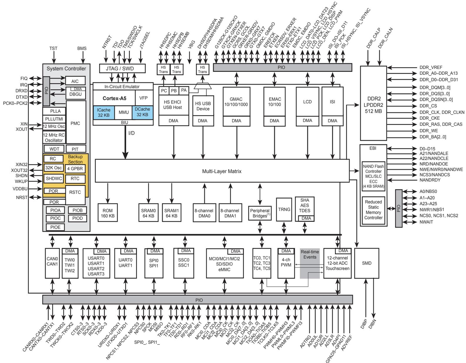
**Note 1:** Peripheral Bridge 0 (APB0) connects HSMCI0, SPI0, USART0, USART1, TWI0, TWI1, UART0, SSC0, SMD.
