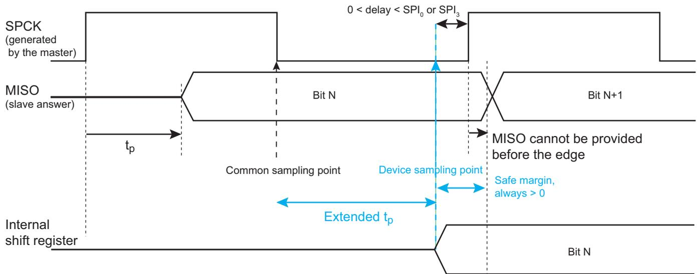
**Figure 54-13: SPI Master Mode 1 and 2**
