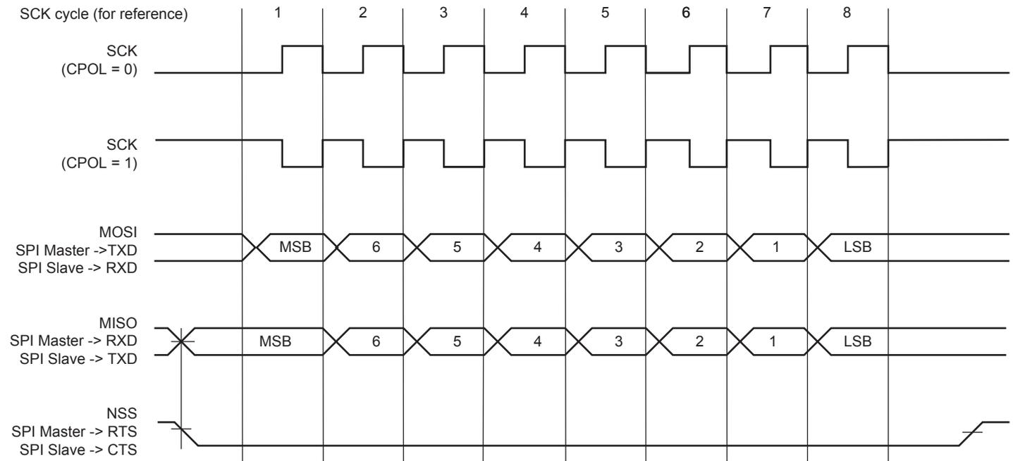
**Figure 44-38: SPI Transfer Format (CPHA = 0, 8 bits per transfer)**
