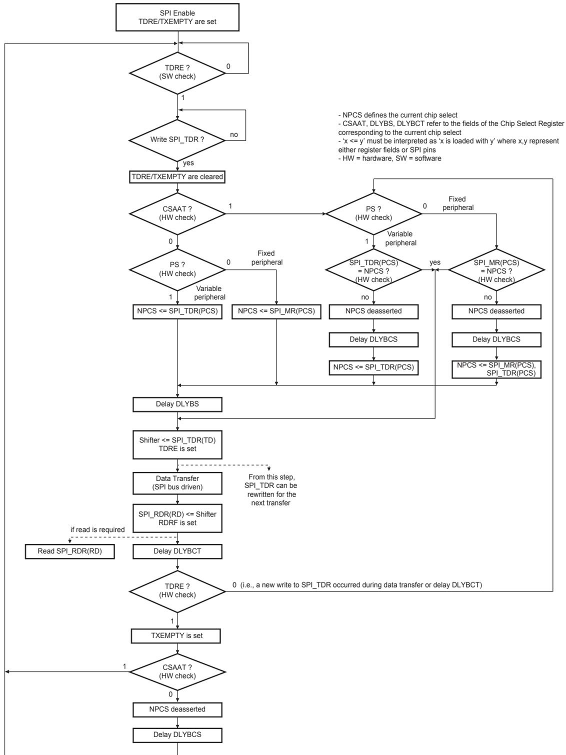
Figure 39-8 shows the behavior of Transmit Data Register Empty (TDRE), Receive Data Register (RDRF) and Transmission Register Empty (TXEMPTY) status flags within the SPI\_SR during an 8-bit data transfer in Fixed mode without the DMA involved.
