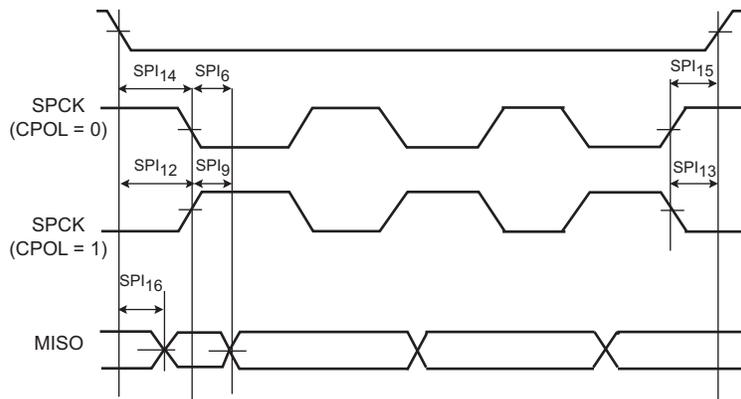
Table 54-52: SPI Timings with 3.3V Peripheral Supply and VDDCORE in [1.08V, 1.32V] Range
