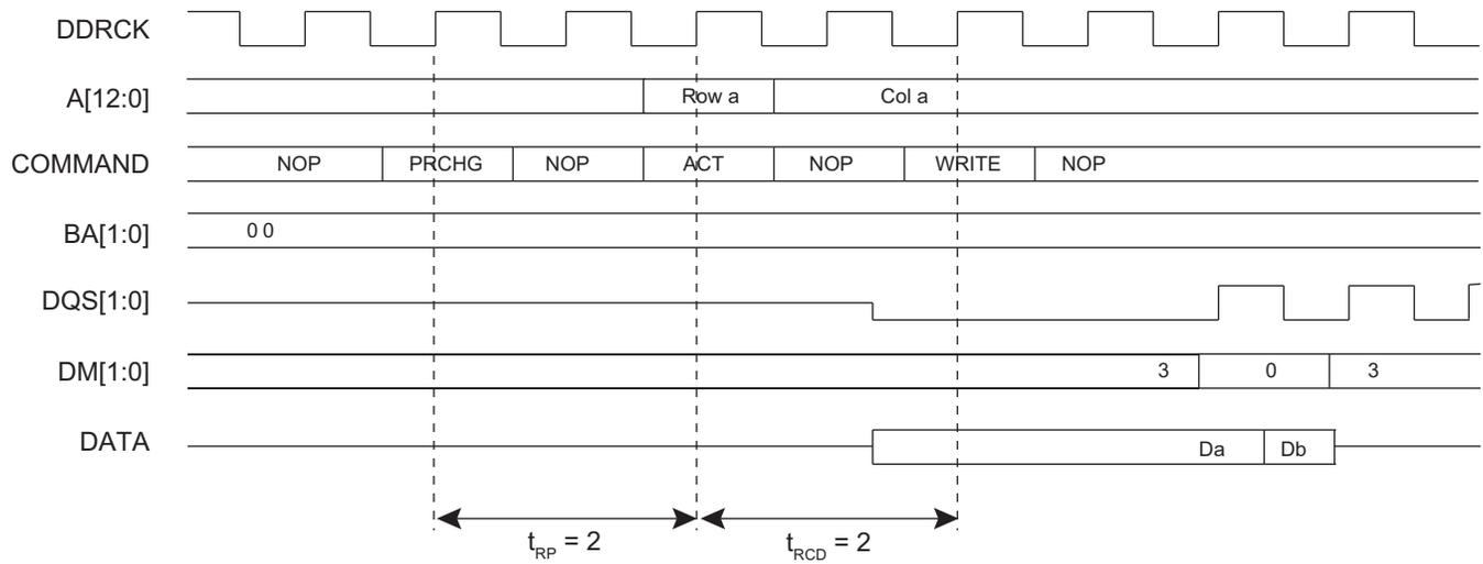
**Figure 29-4: Burst Write Access, Row Closed, DDR-SDRAM Devices**
