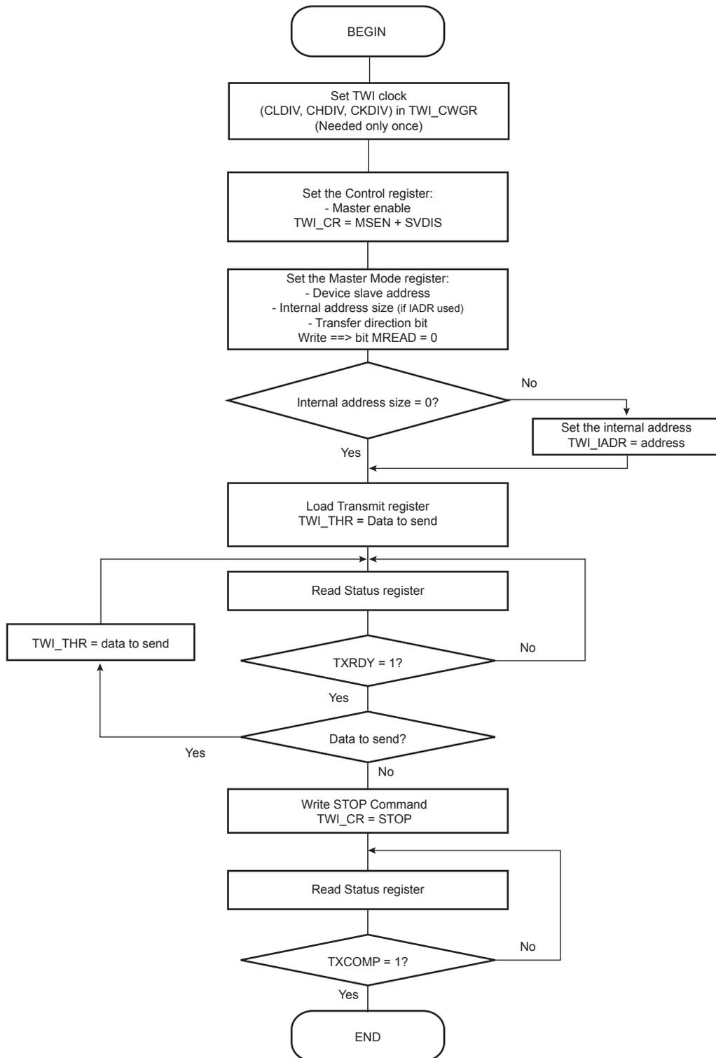
**Figure 40-17: TWI Read Operation with Single Data Byte without Internal Address**
