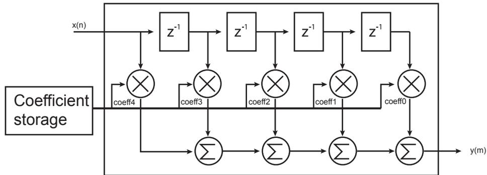
**Figure 32-8: Vertical Resampler Filter Architecture**
