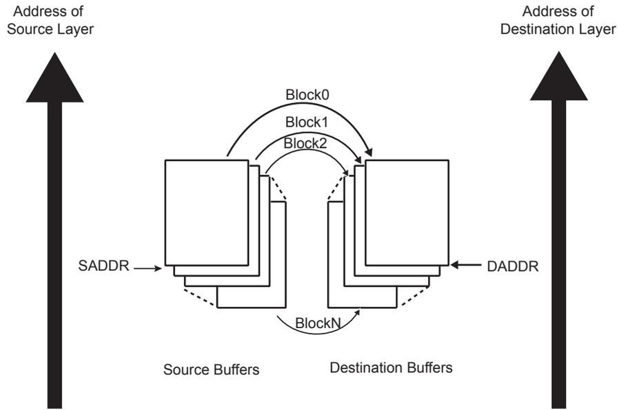
**Figure 31-11: DMAC Transfer Flow for Source and Destination Address Auto-reloaded**
