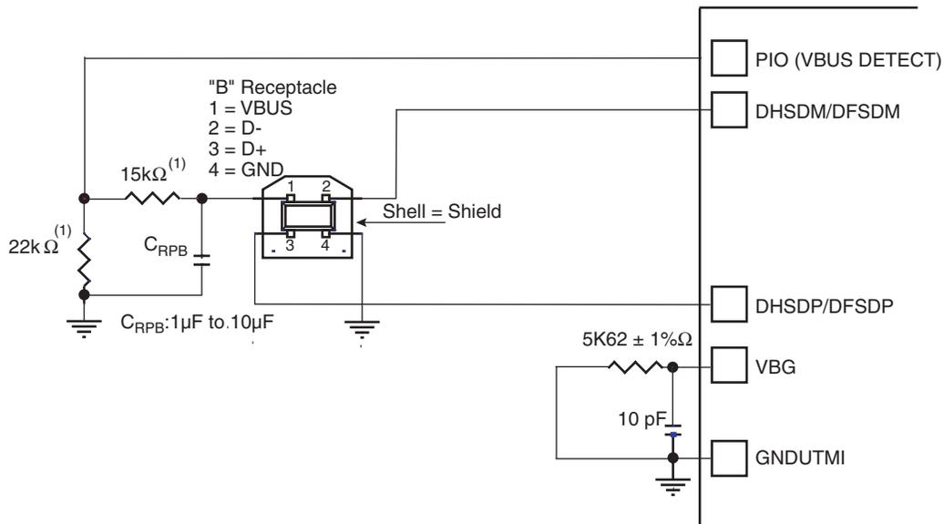
**Note 1:** The values shown on the 22 kΩ and 15 kΩ resistors are only valid with 3.3V supplied PIOs.
