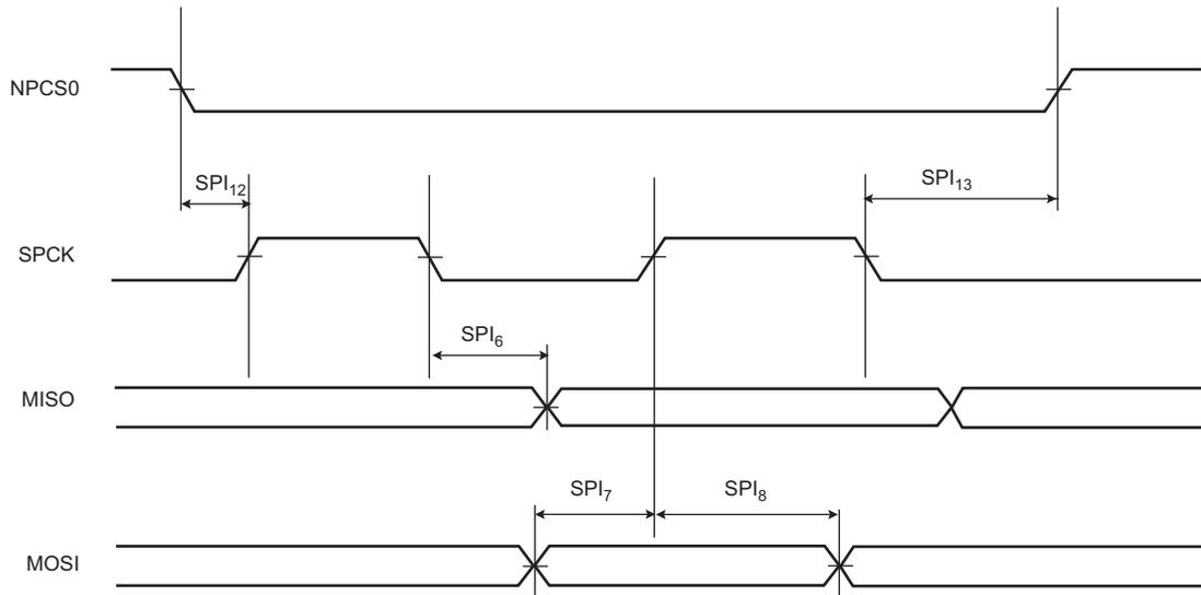
**Figure 54-16: SPI Slave Mode 1 and 2**
