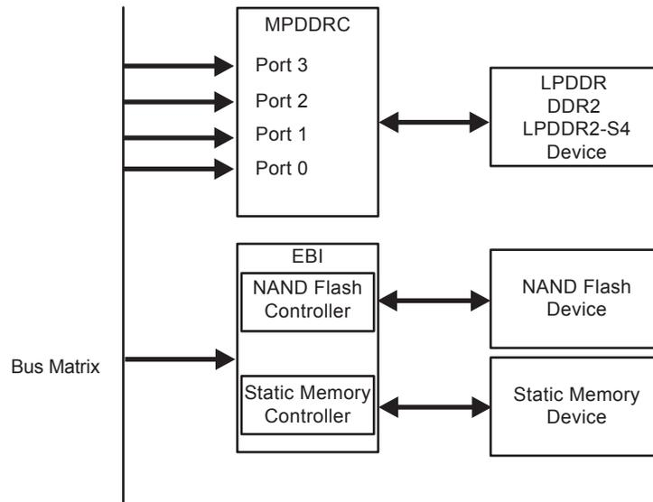
The MPDDRC is a standalone multi-port DDRSDR controller. It supports only 32-bit or 2x16-bit DDR2, LPDDR, and LPDDR2-S4 devices. Its user interface is located at 0xFFFFEA00.
