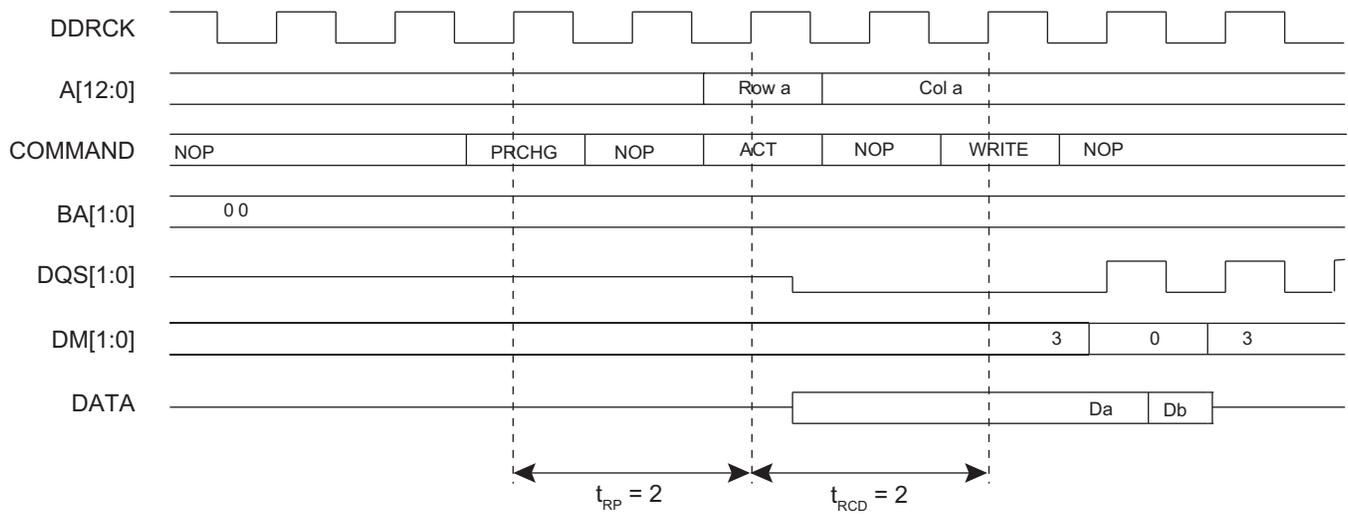
**Figure 29-3: Single Write Access, Row Closed, DDR2-SDRAM Devices**
