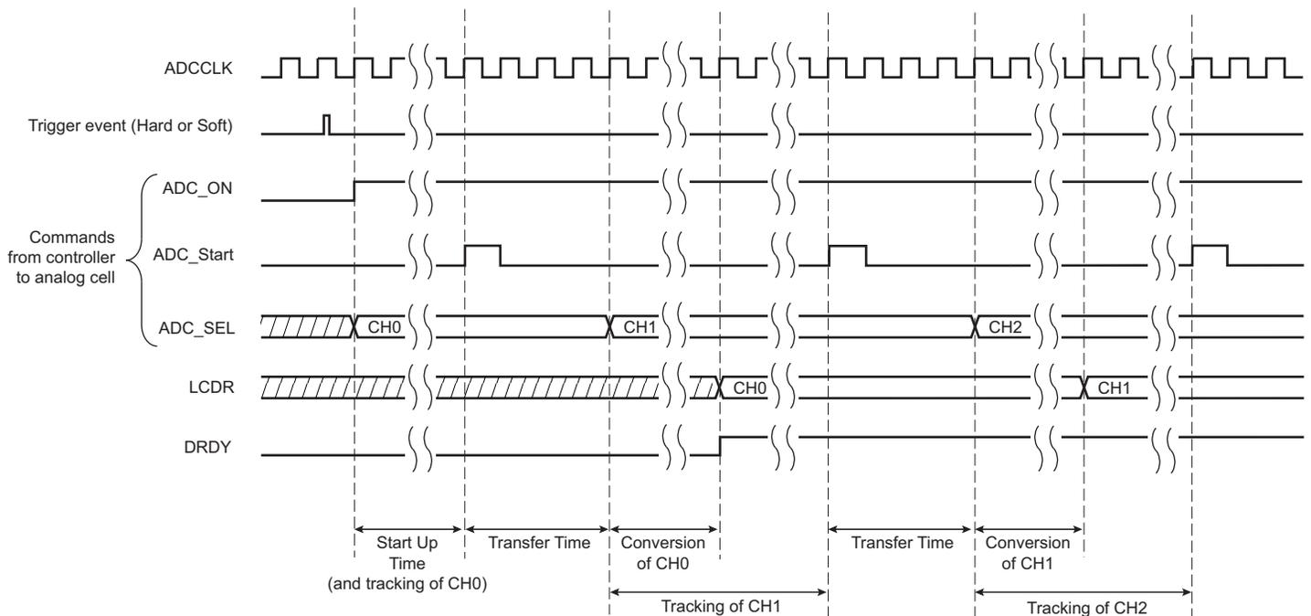
**Figure 49-3: Sequence of ADC Conversions When Tracking Time < Conversion Time**
