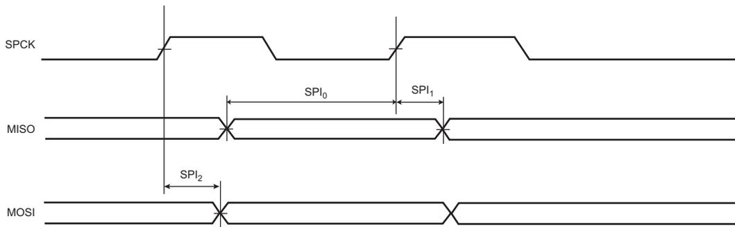
**Figure 54-14: SPI Master Mode 0 and 3**
