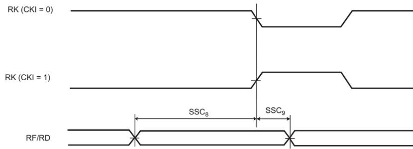
**Figure 54-25: SSC Receiver, RK as Input and RF as Output**
