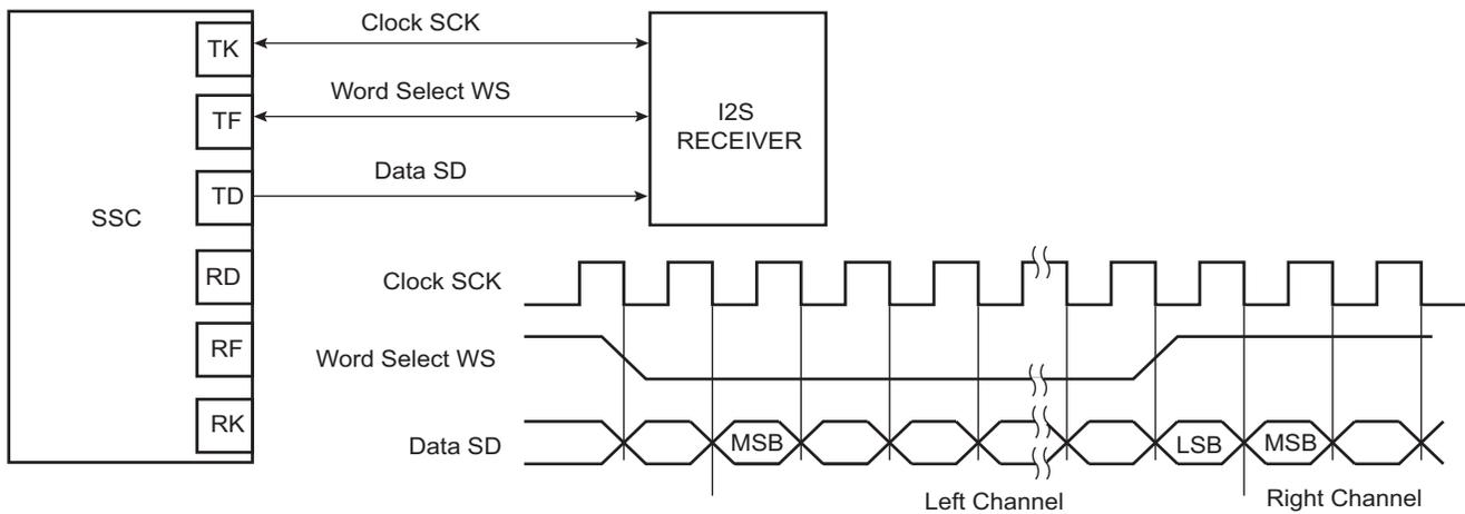
**Figure 41-4: Codec Application Block Diagram**
