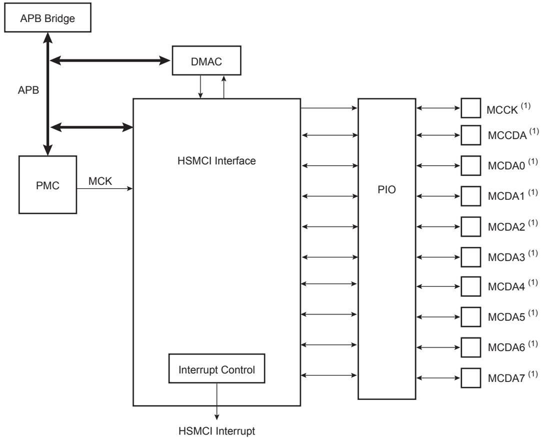
**Note 1:** When several HSMCI (x HSMCI) are embedded in a product, MCCK refers to HSMCI<sub>x</sub>\_CK, MCCDA to HSMCI<sub>x</sub>\_CDA, MCDA<sub>y</sub> to HSMCI<sub>x</sub>\_DA<sub>y</sub>.
