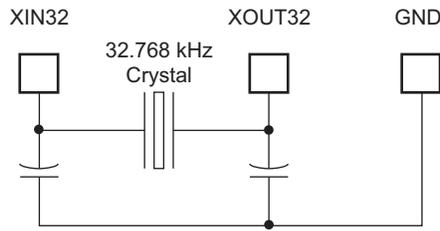
The 32.768 kHz crystal oscillator provides a more accurate frequency than the 32 kHz (typical) RC oscillator.
