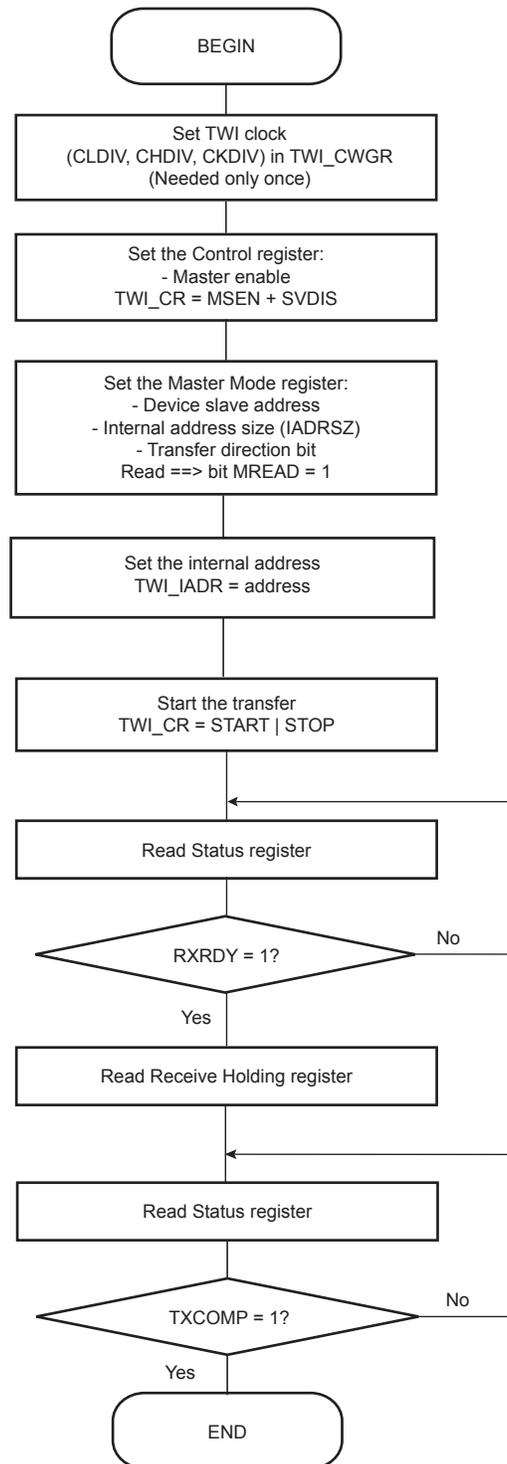
**Figure 40-19: TWI Read Operation with Multiple Data Bytes with or without Internal Address**
