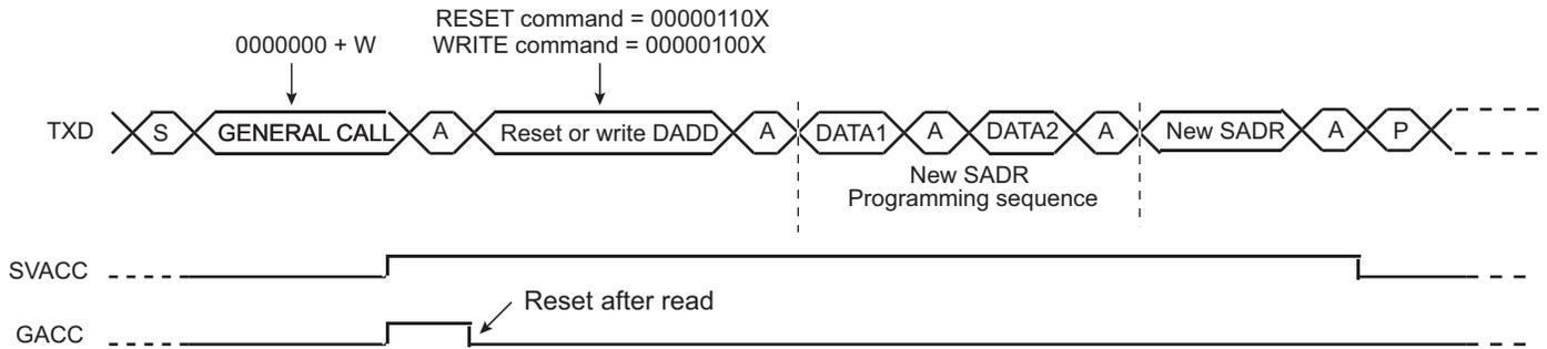
**Note:** This method allows the user to create a personal programming sequence by choosing the programming bytes and the number of them. The programming sequence has to be provided to the master.
