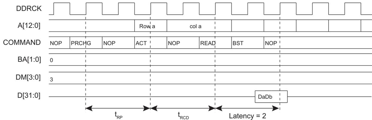
**Figure 29-10: Single Read Access, Row Closed, Latency = 3, DDR2-SDRAM Devices**
