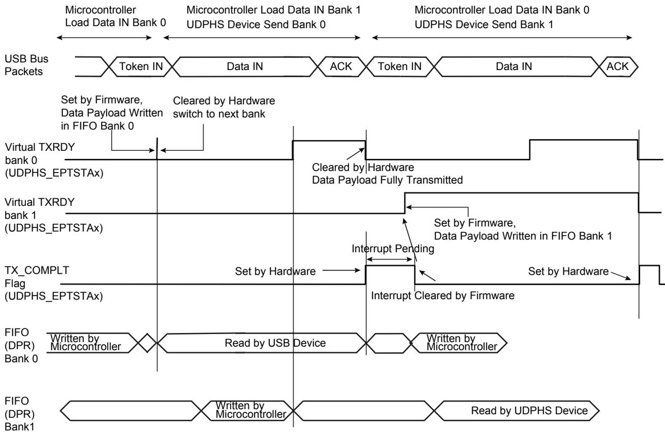
**Figure 34-11: Data IN Followed By Status OUT Transfer at the End of a Control Transfer**
