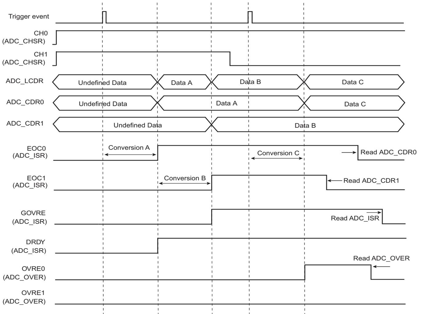
**Warning:** If the corresponding channel is disabled during a conversion or if it is disabled and then reenabled during a conversion, its associated data and corresponding EOCx and GOVRE flags in ADC\_ISR and OVREx flags in ADC\_OVER are unpredictable.
