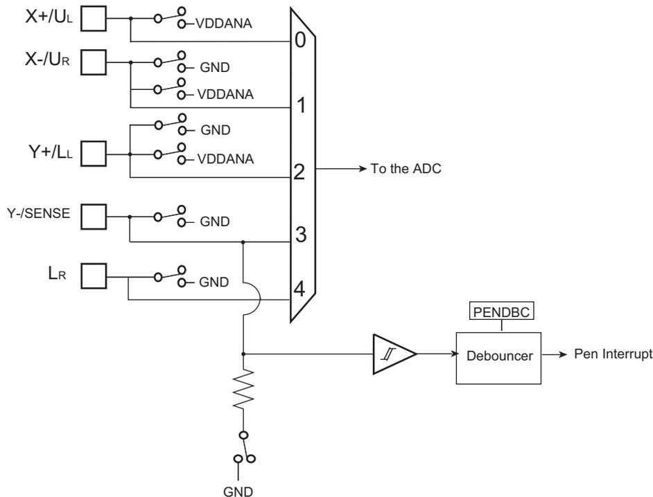
The touchscreen pen detect can be used to generate an ADC interrupt to wake up the system. The pen detect generates two types of status, reported in ADC\_ISR:
