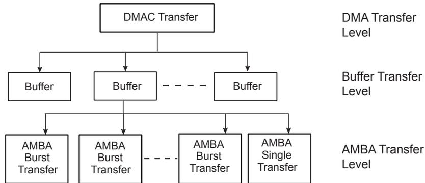
**Buffer:** A buffer of DMAC data. The amount of data (length) is determined by the flow controller. For transfers between the DMAC and memory, a buffer is broken directly into a sequence of AMBA bursts and AMBA single transfers.
