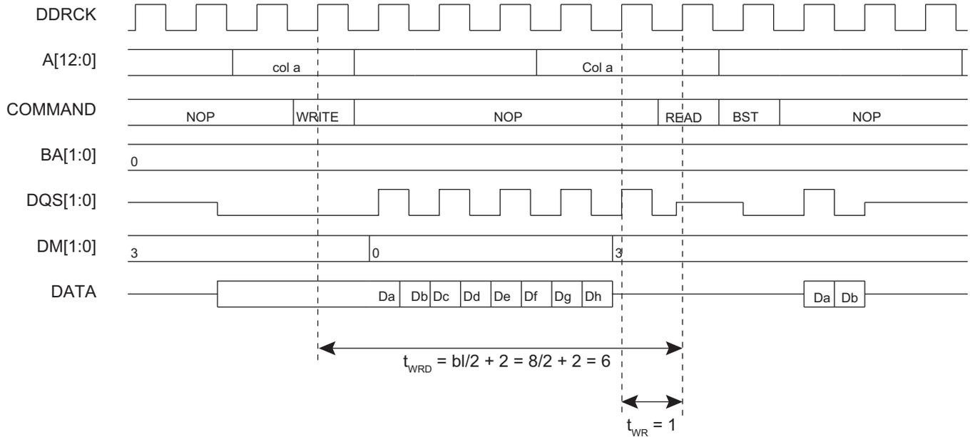
In case of a single write access, write operation should be interrupted by a read access but DM must be input 1 cycle prior to the read command to avoid writing invalid data. See [Figure 29-7](#).
