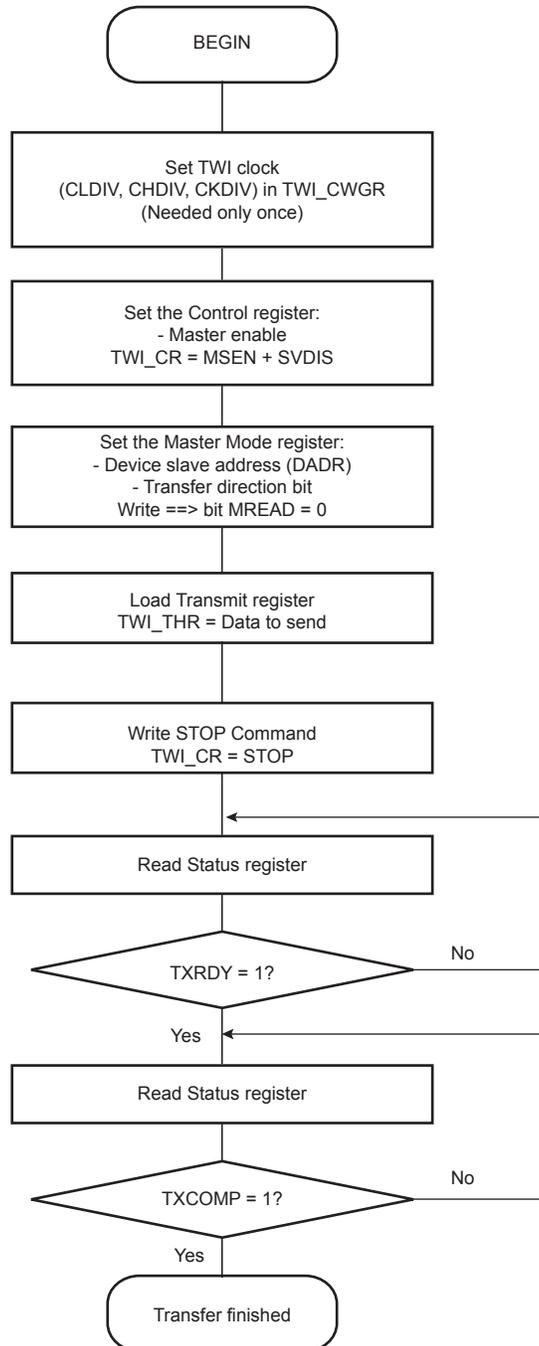
Figure 40-15: TWI Write Operation with Single Data Byte and Internal Address
