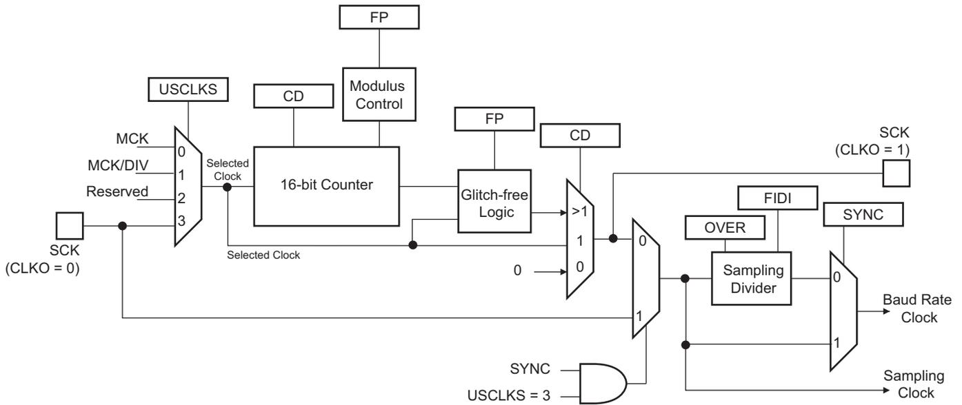
**Warning:** When the value of field FP is greater than 0, the SCK (oversampling clock) generates non-constant duty cycles. The SCK high duration is increased by “selected clock” period from time to time. The duty cycle depends on the value of the CD field.
