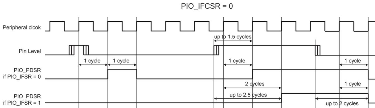
**Figure 27-5: Input Debouncing Filter Timing**
