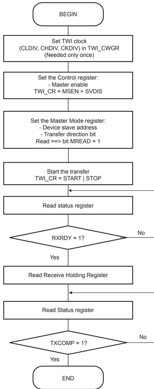
Figure 40-18: TWI Read Operation with Single Data Byte and Internal Address
