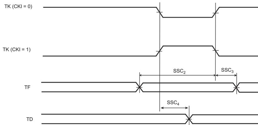
**Figure 54-23: SSC Transmitter, TK and TF in Input**
