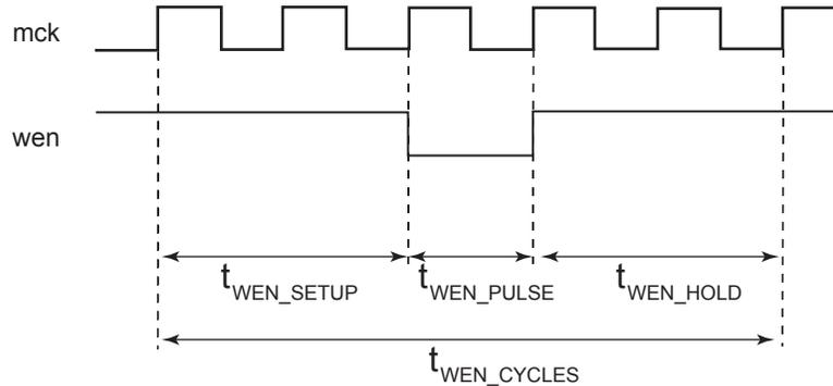
**Figure 30-33: Write Enable Timing for NAND Flash Device Data Input Mode**
