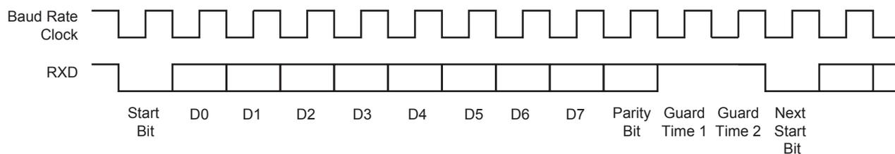
**Figure 44-31: T = 0 Protocol with Parity Error**
