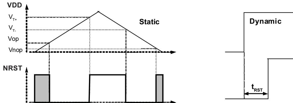
When a very slow (versus  $t_{RST}$ ) supply rising slope is applied on the POR VDD pin, the reset time becomes negligible and the reset signal is released when  $V_{DD}$  rises higher than  $V_{T+}$ .
