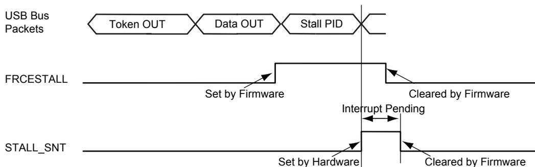
**Figure 34-18: Stall Handshake Data IN Transfer**
