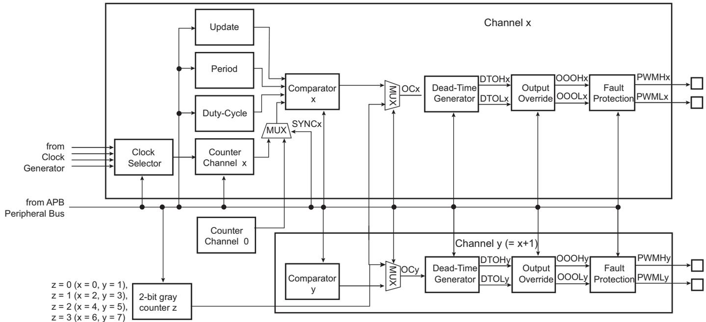
Each of the 4 channels is composed of six blocks:
