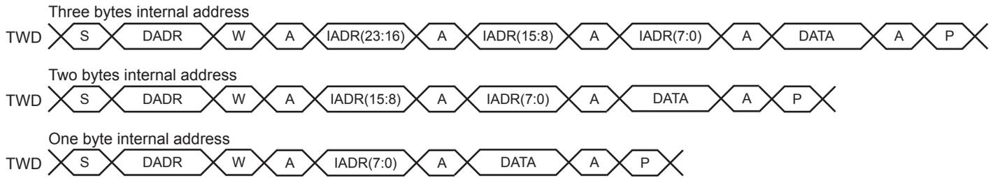
**Figure 40-11: Master Read with One, Two or Three Bytes Internal Address and One Data Byte**
