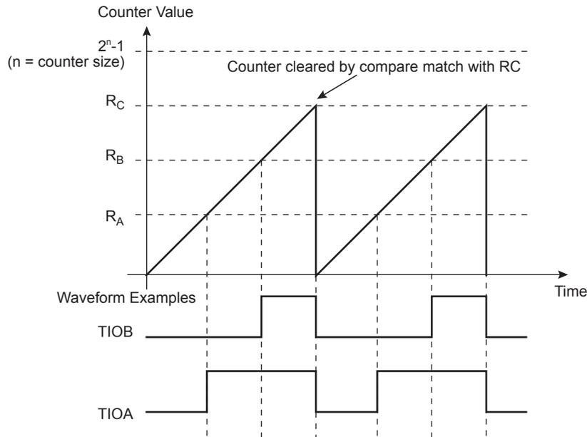
**Figure 47-10: WAVSEL = 10 with Trigger**
