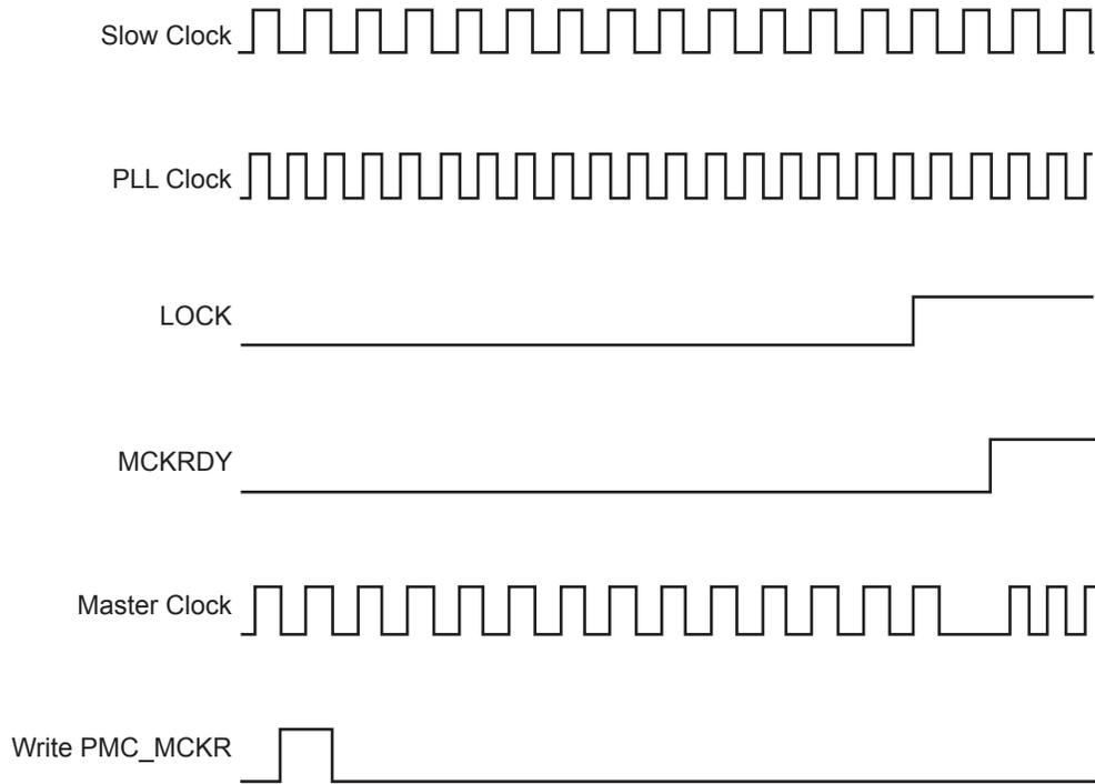
**Figure 26-7: Switch Master Clock from Main Clock to Slow Clock**
