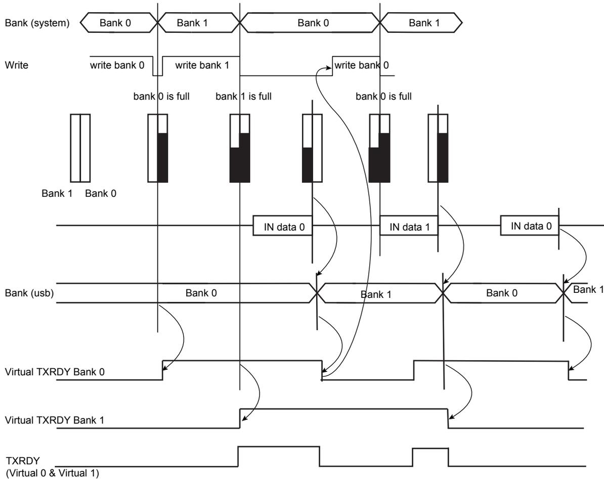
**Note:** In the illustration above Autovalid validates a bank as full, although this might not be the case, in order to continue processing data and to send to DMA.
