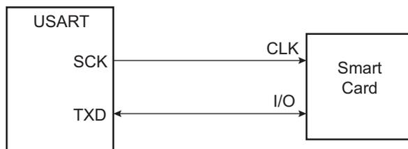
When operating in ISO7816, either in T = 0 or T = 1 modes, the character format is fixed. The configuration is 8 data bits, even parity and 1 or 2 stop bits, regardless of the values programmed in the CHRL, MODE9, PAR and CHMODE fields. MSBF can be used to transmit LSB or MSB first. Parity Bit (PAR) can be used to transmit in Normal or Inverse mode. Refer to [Section 44.7.3 USART Mode Register and PAR: Parity Type](#).
