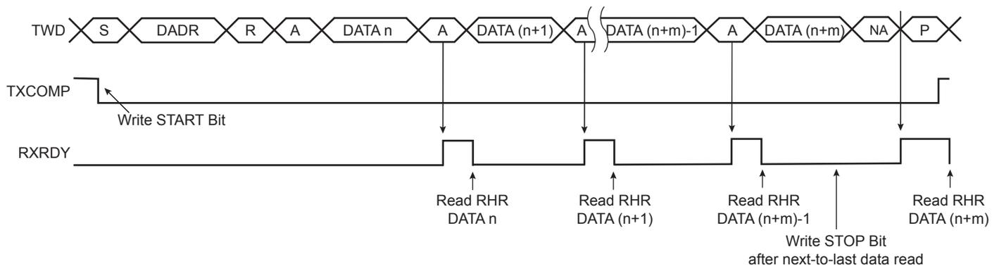
**Figure 40-9: Master Read Wait State with Multiple Data Bytes**
