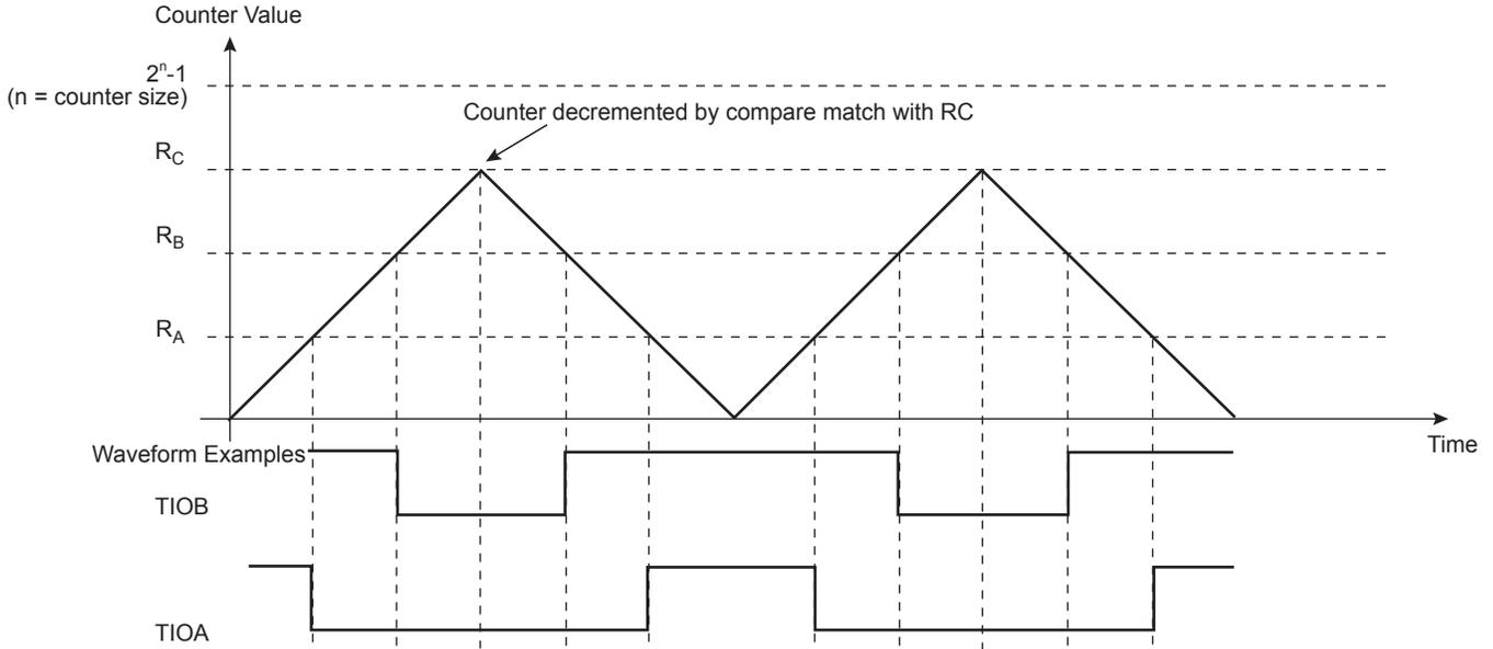
**Figure 47-14: WAVSEL = 11 with Trigger**
