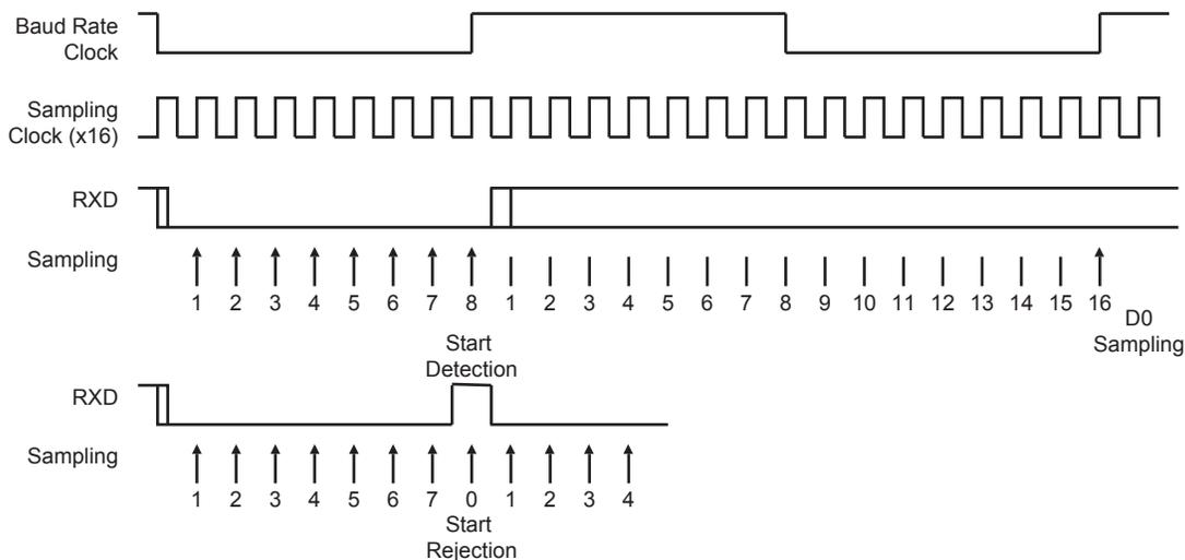
**Figure 44-12: Asynchronous Character Reception**
