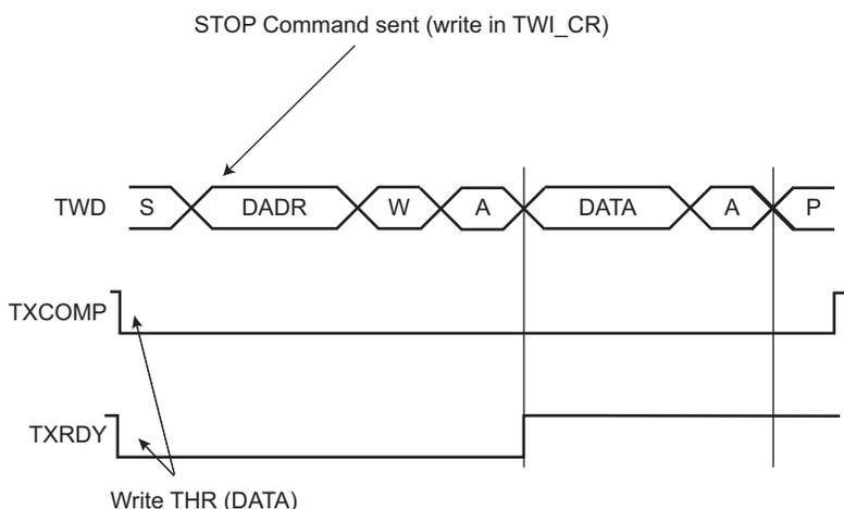
**Figure 40-5: Master Write with Multiple Data Bytes**
