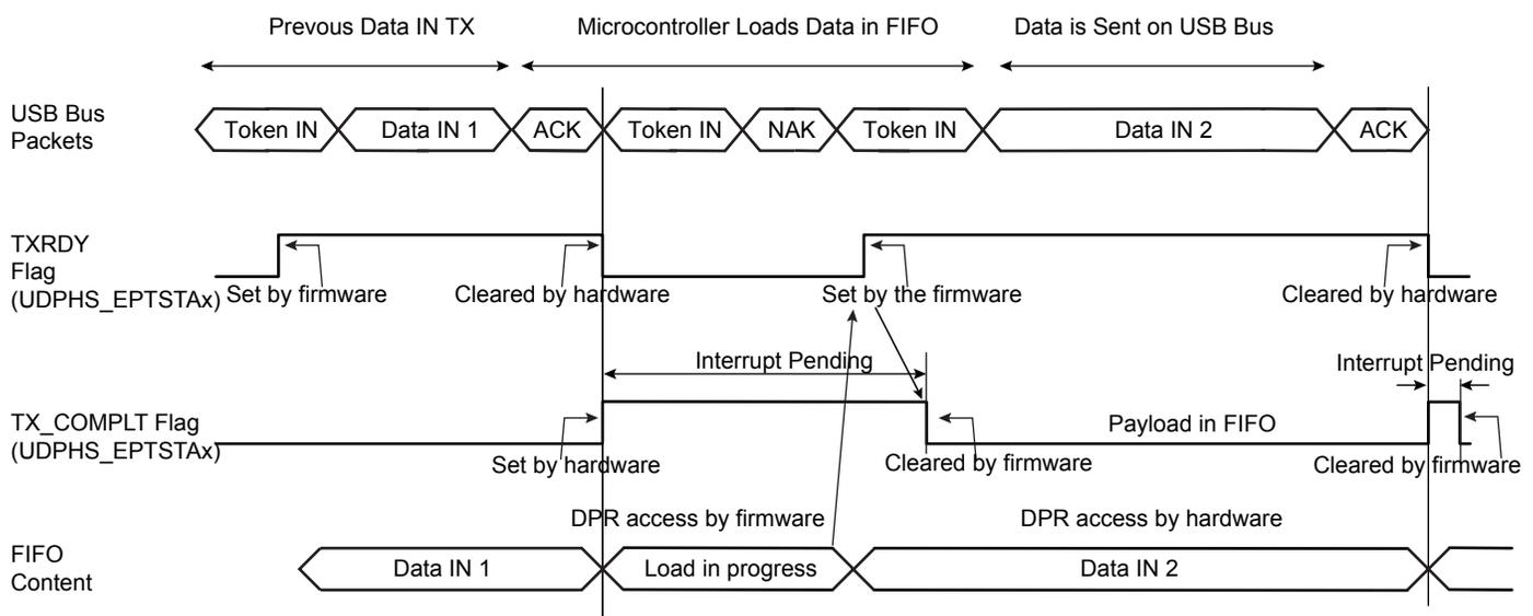
**Figure 34-10: Data IN Transfer for Endpoint with Two Banks**
