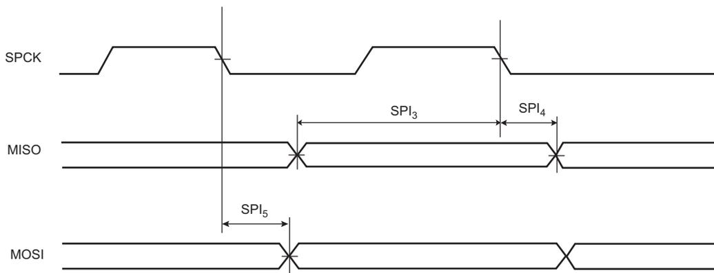
**Figure 54-15: SPI Slave Mode 0 and 3**
