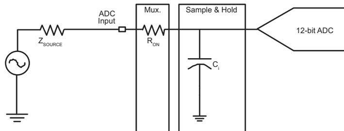
In 12-bit mode, during the tracking phase, the ADC must track the input signal during the tracking time shown below:
