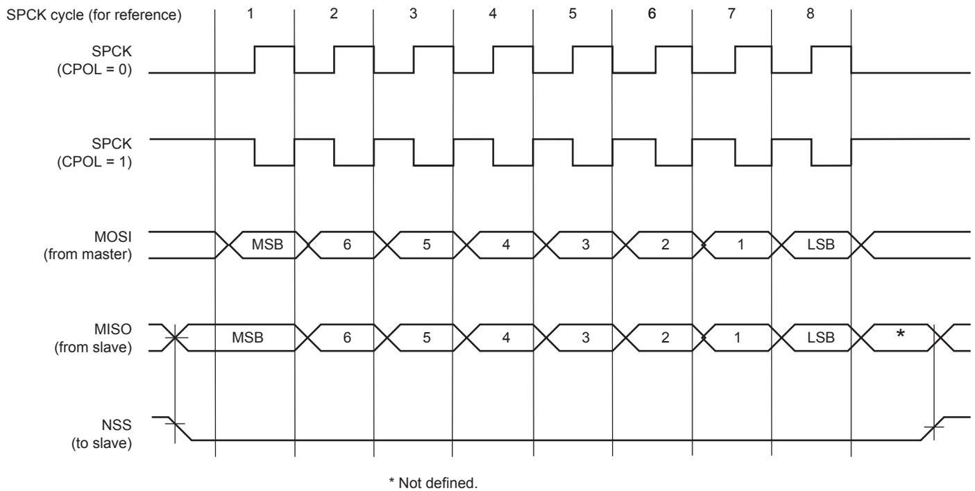
**Figure 39-4: SPI Transfer Format (NCPHA = 0, 8 bits per transfer)**
