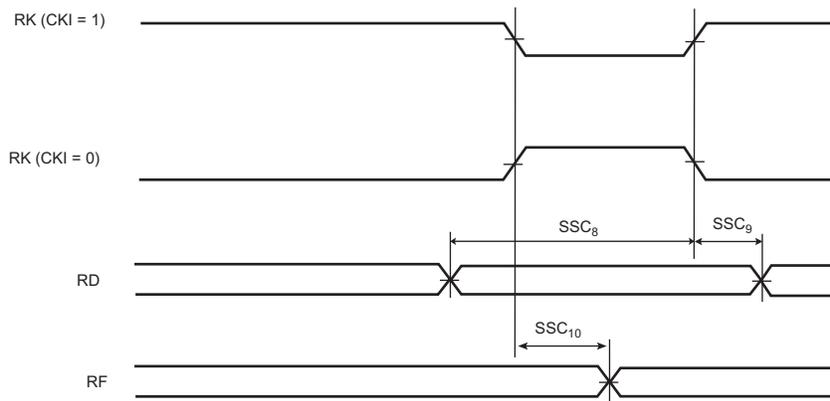
**Figure 54-26: SSC Receiver, RK and RF as Output**
