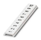
Zack Marker strip, flat, Strip, white, labeled, printed horizontally: consecutive numbers 1 ... 10, 11 ... 20, etc. up to 91 ... 100, mounting type: snapped, for terminal block width: 3.5 mm, lettering field size: 5.15 x 3.5 mm, Number of individual labels: 10
