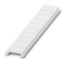
Zack Marker strip, flat, can be ordered: Strip, white, labeled according to customer specifications, mounting type: snap into flat marker groove, for terminal block width: 3.5 mm, lettering field size: 3.5 x 5.2 mm, Number of individual labels: 10
