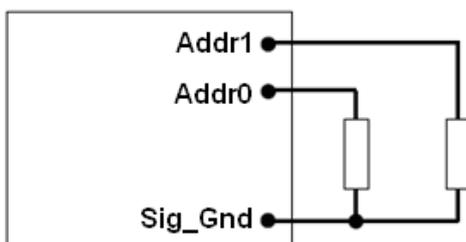
Corresponded to each octal digit, the requested resistor values are shown in below, and +/-1% resistors accuracy can be accepted. If there are any resistances exceeding the requested range, address 127 will be return. 0-12 and 40, 44, 45, and 55 in decimal address can't be used, since they are reserved according to the SMBus specifications, and which will also return address 127. The address resistance will be considered as 200k if resistor  $\geq 200k$ .
