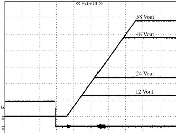
**Figure 4: Remote On/Off (negative logic) at no load**
