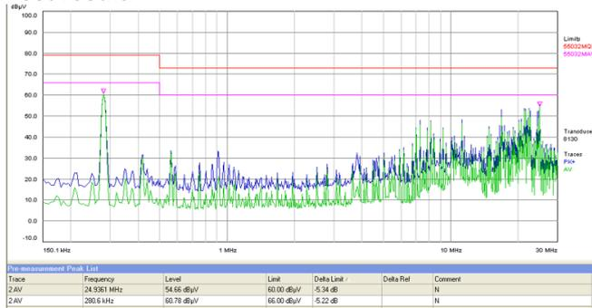
Short CASE to Ground in EMC test
