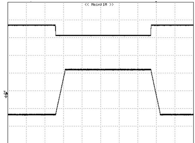
**Figure 7: Output Voltage vs. Vset pin voltage dynamic;**
