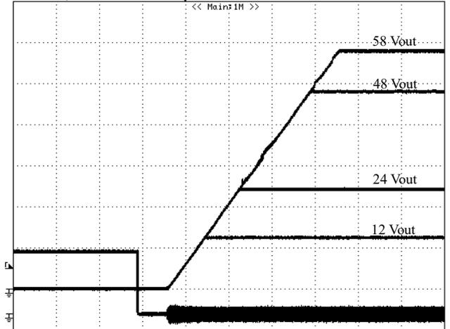
**Figure 5: Remote On/Off (negative logic) at full load**
