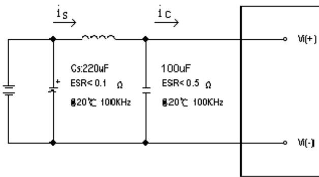
**Figure 10: Test Setup Diagram for Input Ripple Current**
