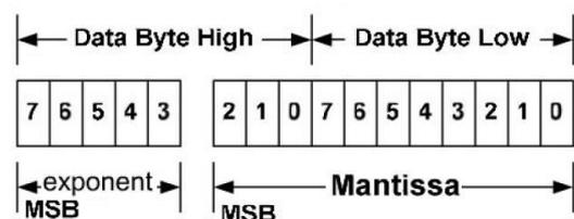
For example, considering set the turn on threshold of input under voltage lockout to 34V by VIN\_ON command; the read/write data can be calculated refer to below process:
