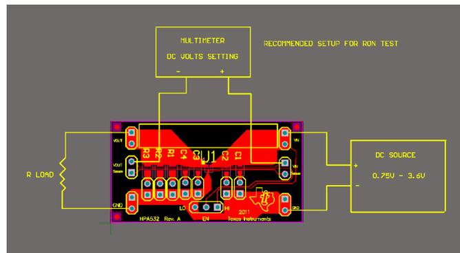
Figure 1.  $r_{ON}$  Setup
