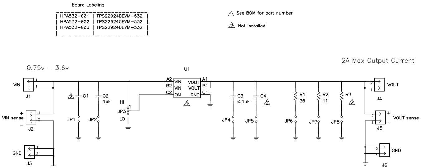
Figure 5. TPS22924EVM-532 Schematic
