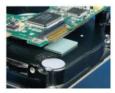
Gap Pad 2200SF is a thermally conductive, electrically isolating, silicone-free polymer specially designed for silicone-sensitive applications. The material is ideal for applications with uneven topologies and high stackup tolerances. Gap Pad 2200SF is reinforced for easy material handling and added durability during assembly. The material is available with a protective liner on both sides. Gap Pad 2200SF is supplied with reduced tack on one side allowing for burn-in processes and easy rework.
