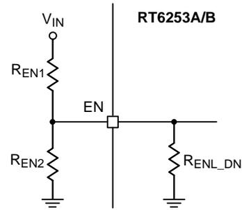
Figure 9. Resistor Divider for Lockout Threshold Setting
