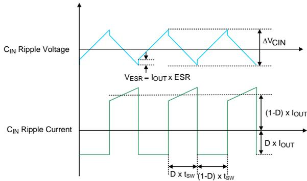
Figure 1. C<sub>IN</sub> Ripple Voltage and Ripple Current
