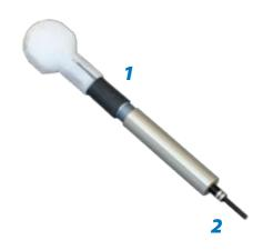
Check for properly seated contacts with this spring-loaded tester. Apply the tool tip to the mating end of a contact. Push on the handle until the spring compresses to the recommended force. A visual indicator shows full compression. The contact is properly retained if it is not displaced.
