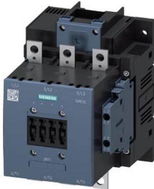
Power contactor, AC-3 185 A, 90 kW / 400 V AC (50-60 Hz) / DC operation
