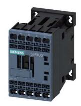
Power contactor, AC-3 12 A, 5.5 kW / 400 V 2 NO + 2 NC 220 V DC, 50 Hz 240 V, 60 Hz 4-pole Size S00 Spring-type terminals
