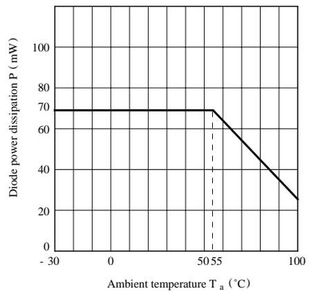
**Fig. 3 Collector Power Dissipation vs. Ambient Temperature**
