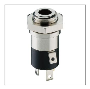
Jack chassis socket according to JEITA RC-5325A JC35C4A, 3.5 mm, 4 poles/stereo, upright version, with solder eyes, for back side mounting
