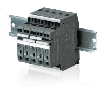
The protection devices EPD24 extend the ABB product range of Modular DIN Rail Components by electronic overcurrent protection modules for selective protection of 24 V DC load circuits. This protection is achieved by a combination of active electronic current limitation in the case of a short circuit and an overload deactivation from 1.1 x  $I_N$  upwards.
