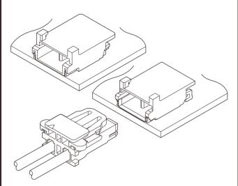
Board-to-wire connector with high withstanding voltage, used for power supply of LCD (Liquid Crystal Display) back light.
