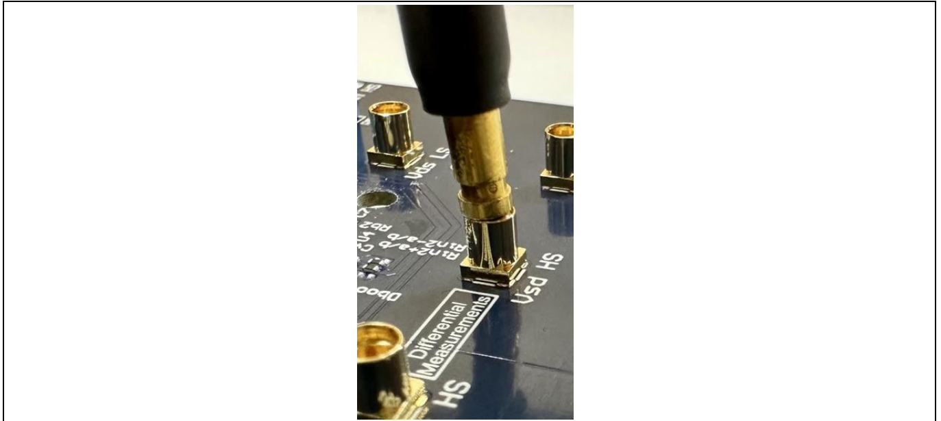
Figure 13 High-side differential voltage measurements with high-bandwidth differential probes
