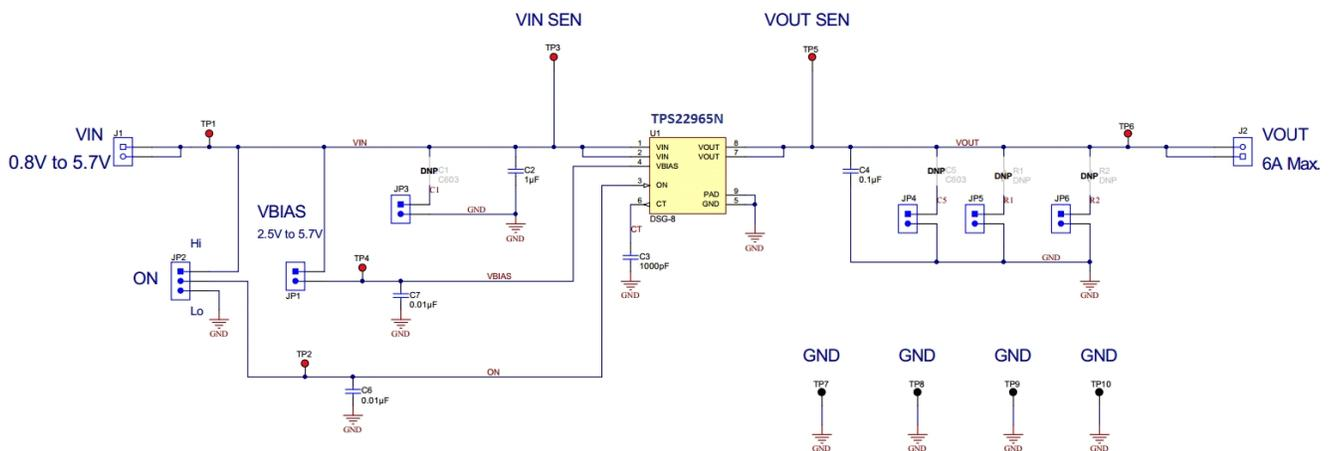
Figure 2. TPS22965NEVM Schematic
