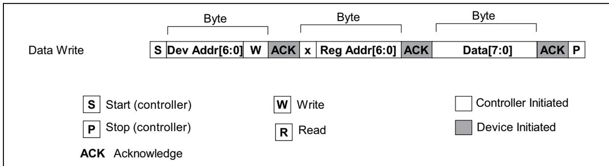
**FIGURE 7-5:** I<sup>2</sup>C Data Write Protocol.
