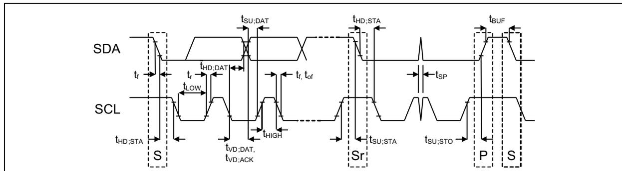
**FIGURE 9-4:** I<sup>2</sup>C Interface Timing.
