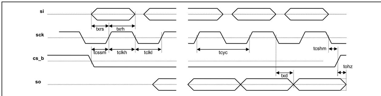
**FIGURE 9-3: SPI Interface Timing, MSB First Mode.**
