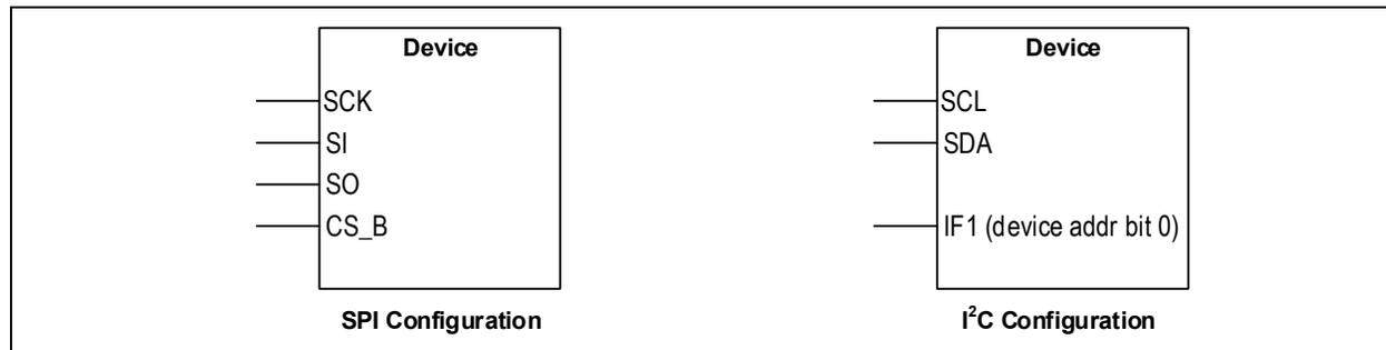
**FIGURE 7-1:** Host Interface Pins for SPI and I<sup>2</sup>C.
