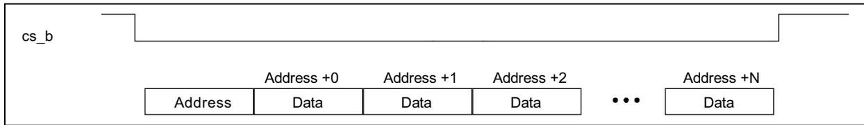
**FIGURE 7-4:** Example of the Burst Mode Operation.
