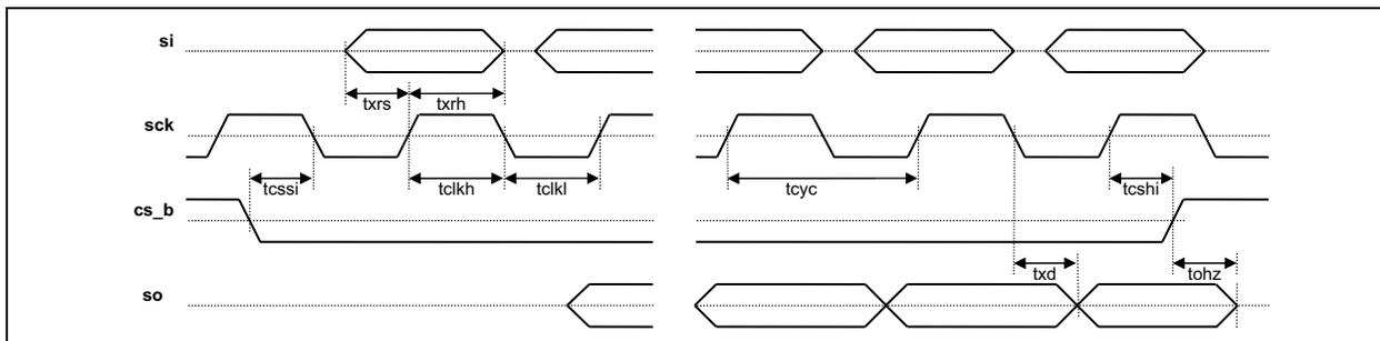
**FIGURE 9-2: SPI Interface Timing, LSB First Mode.**
