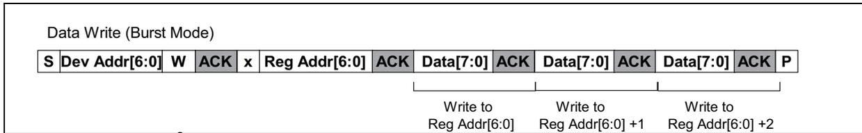
**FIGURE 7-8:** *I<sup>2</sup>C Data Write Burst Mode.*
