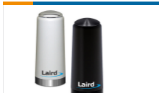
TE Part #TRA6927M3NW-001 OMNI,Ph,NMO,698/1710 MHz WHT,3 dBi,100W,
