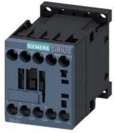
Contactor relay, 3 NO + 1 NC, 24 V DC, Size S00, screw terminal Upright mounting position  $\,$
