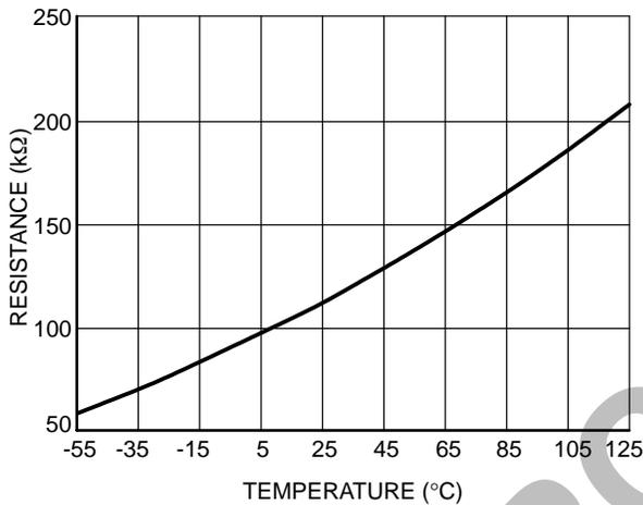
Figure 1. MC623 Sense Resistors vs. Trip Temperature
