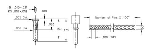
**Description:** Interconnect Carrier Plastic Carrier with Ultra Low Profile Receptacles Single Row Through Hole Plating Code: 93 Shell Plating: 200 μ" Tin/Lead(93/7) over 100 μ"
