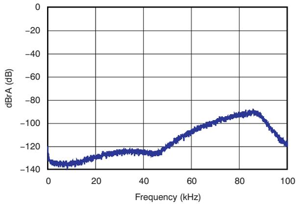
**Figure 11. Idle Noise FFT Spectrum (Digital Input)**
