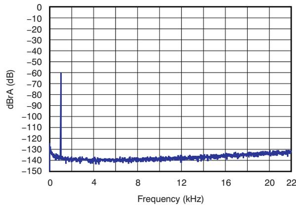
**Figure 9. FFT Spectrum with -60-dBFS Tone (Digital Input)**
