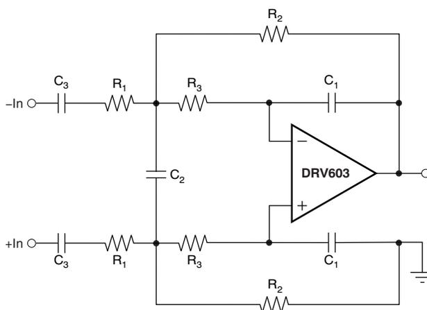
**Figure 3. Differential Input, Second-Order, Active Low-Pass Filter**
