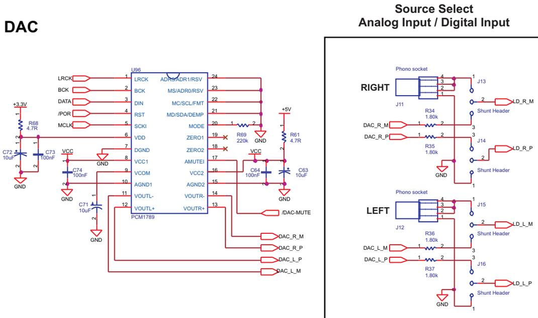
Figure 19. DRV603EVM Schematic: Digital-to-Analog Converter and Source Select
