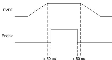
**Figure 2. Power-Up/-Down Sequence**
