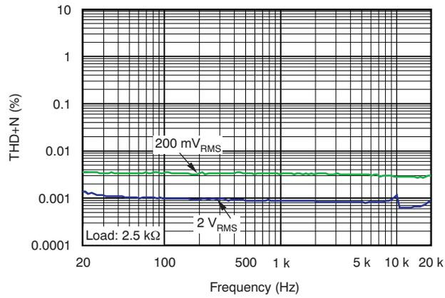
Figure 6. THD+N versus Frequency (Analog Input)
