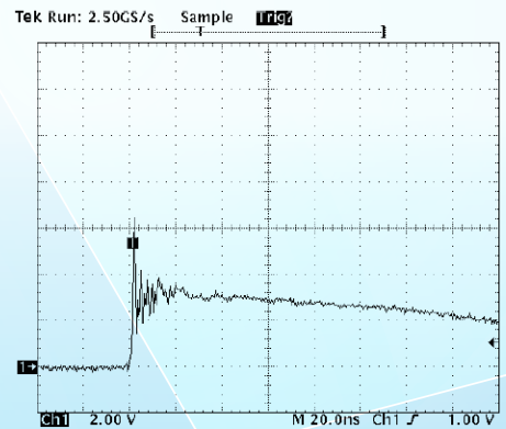
ESD Clamping Voltage 8 kV Contact per IEC61000-4-2
