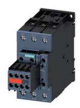
Contactor, AC-3, 30 kW / 400 V, 2 NO + 2 NC, 110 V AC, 50 Hz / 120 V, 60 Hz, 3-pole, Size S2, screw terminal captive auxiliary switch block
