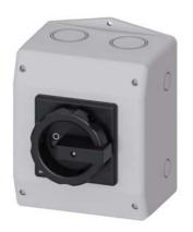
SENTRON, Switch disconnector 3LD, main switch, 6-pole, lu: 25 A, Operating power / at AC-23 A at 400 V: 9.5 kW, molded-plastic encapsulation for metric screw connection, 1 NC, 1 NO, rotary operating mechanism, black
