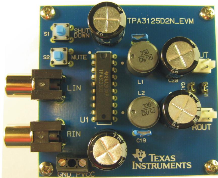
Figure 2. TPA3125D2 Audio Power Amplifier EVM - Bottom View
