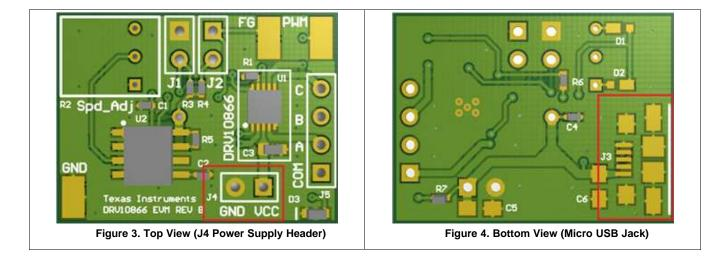
**NOTE:** It is only necessary to provide one source of power for the EVM. DO NOT connect to both the micro USB jack and the J4 power supply header.
