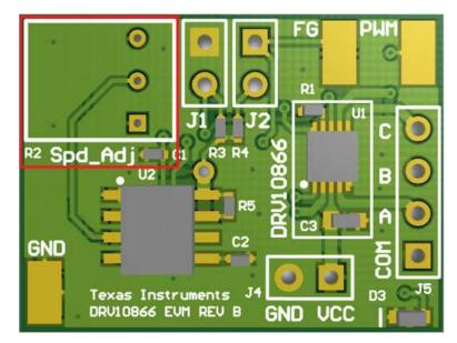
Figure 8. Speed Adjust Potentiometer
