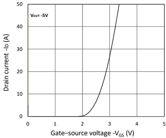
Figure 2. Transfer Characteristics
