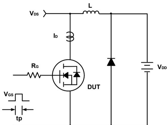
Figure C. Unclamped Inductive Switching Circuit & Waveforms
