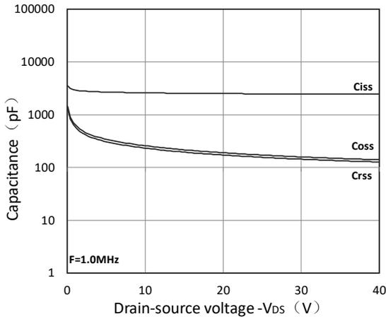
Figure 7. Capacitance Characteristics
