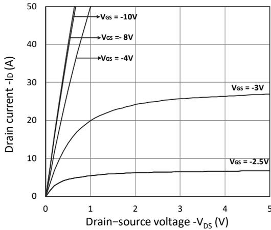
Figure 1. Output Characteristics
