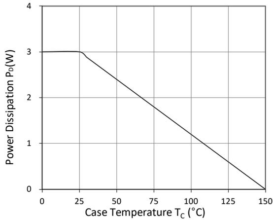
Figure 9. Power Dissipation
