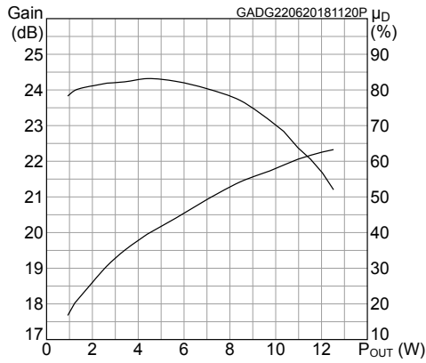
Figure 1. Power gain and efficiency versus output power ( f = 930\text{MHz} , V_{DD} = 28\text{V} , I_{DQ} = 0.1\text{A} )
