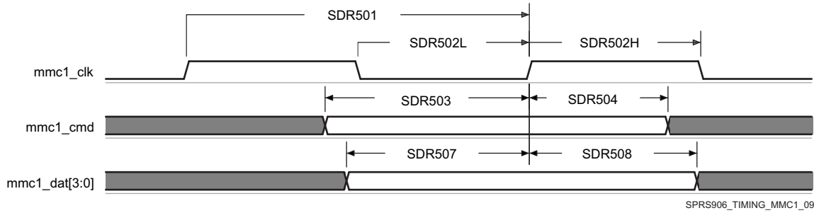
Figure 7-69. MMC/SD/SDIO in - High Speed SDR50 - Receiver Mode
