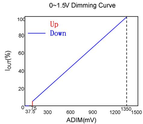
Fig.11 Dimming curve of analog dimming
