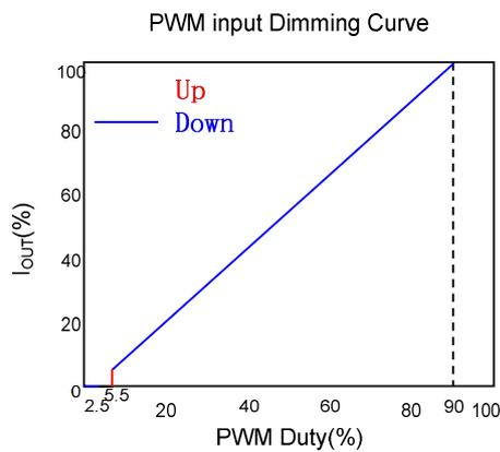
Fig.13 the dimming curve of PWM input
