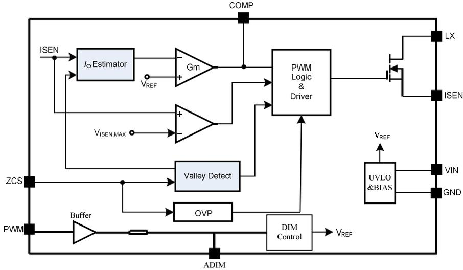
Figure.3 Block Diagram
