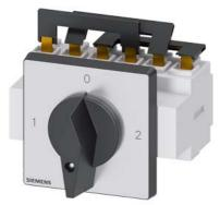
SENTRON, Switch disconnector 3LD, change-over switch, 3-pole, lu: 63 A, Operating power / at AC-23 A at 400 V: 22 kW, front-mounted, knob-operated mechanism, black, 4-hole mounting of the handle
