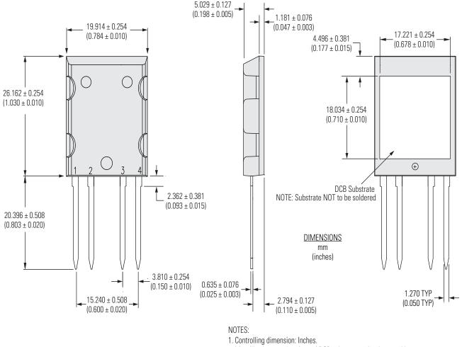
2. Metallized external surface of DCB substrate maintains 2500V  $_{\rm rms}$
