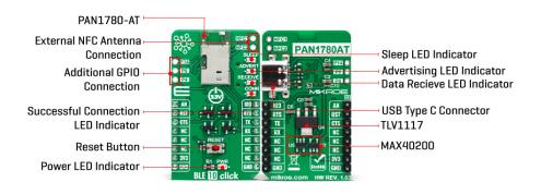
The Bluetooth® 5 features an additionally higher symbol rate of 2Mbps using the high-speed LE 2M PHY or a significantly longer range using the LE Coded PHY. The output power of up to 8dBm and the high sensitivity of the nRF52840 combined with the LE Coded PHY make this module very attractive in long-range applications.
