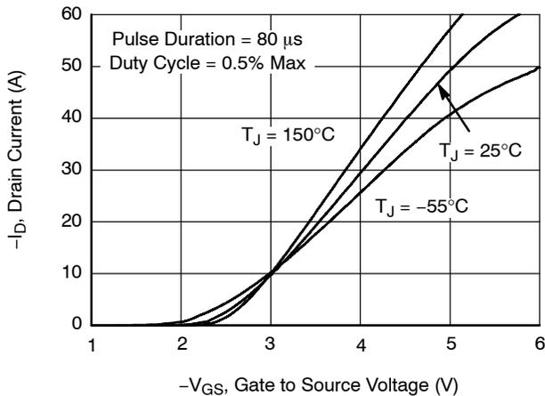
Figure 5. Transfer Characteristics
